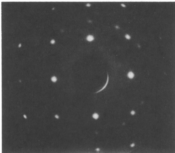
FIG. 10. LEED pattern for the graphite-covered TaC(001). E_0 = 227.1 eV.
