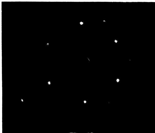
FIG. 8. LEED pattern for the graphite-covered TiC(111). Only one domain can be seen. Primary energy was 202.3 eV.
