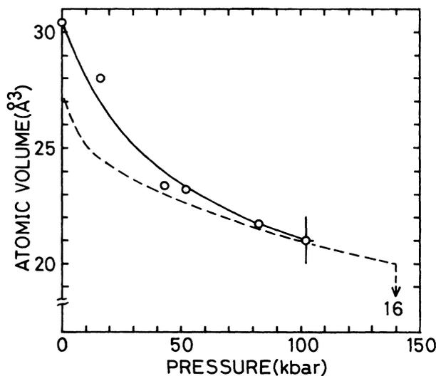
FIG. 2. Pressure dependences of the atomic volume in *a*-Se (open circles with solid line) and hexagonal Se (dashed line). The error bars attached to the 103-kbar point apply to other experimental points. The hexagonal form undergoes a phase transition to a monoclinic form with an atomic volume of  $16 \text{ \AA}^3$  at 140 kbar.
