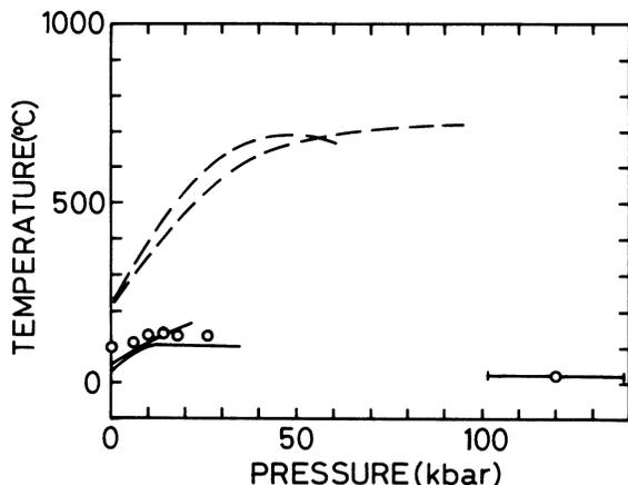
FIG. 3. The pressure dependence of the melting temperature  $T_m$  (dashed line), the crystallization temperature  $T_c$  (open circles), and the glass-transition temperature  $T_g$  (solid line). An error bar is attached for the  $T_c$  datum at 120 kbar. For references of  $T_m$  and  $T_g$ , see the text.
