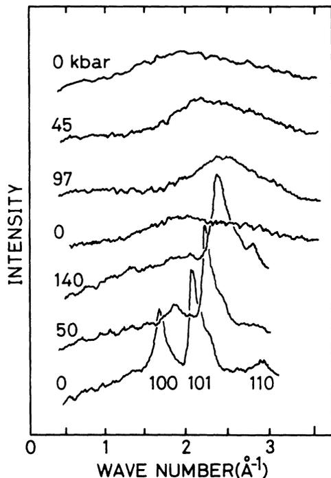
FIG. 1. X-ray-diffraction patterns in *a*-Se under compression. The pressure is changed successively from the upper plot to the lower one. The intensity scale of crystalline samples is reduced to one-half of the amorphous scale. Peak indices in the hexagonal representation are given for the bottom pattern.
