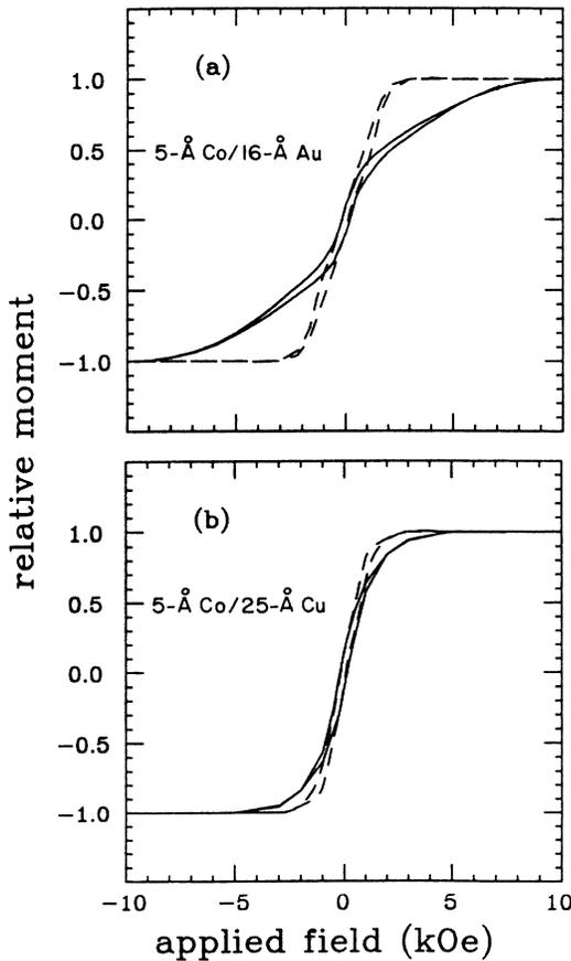
FIG. 1. Hysteresis loops of (a) 5-Å Co-16-Å Au and (b) 5-Å Co-25-Å Cu superlattices measured at 300 K with the applied magnetic field parallel (solid curves) and perpendicular (dashed curves) to the film plane.
