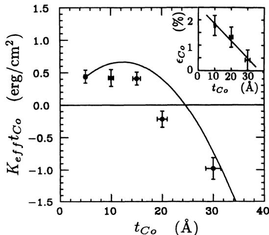
FIG. 2. Measured (points) and calculated anisotropies for a series of Co-Au superlattices. The calculation (solid curve) employed the Co-layer strains given by the linear fit to the measured strains shown in the inset. The magnetocrystalline anisotropy and magnetoelastic constants used here are those of hcp Co.
