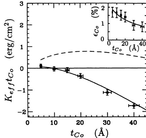
FIG. 3. Measured (points) and calculated anisotropies for a series of Co-Cu superlattices. One calculation (dashed curve) was performed using the magnetocrystalline anisotropy and magnetoelastic constants of hcp Co. The second calculation (solid curve) was performed with modified constants, as described in the text. Both calculations employed the Co-layer strains given by the fit to the measured strains (inset).
