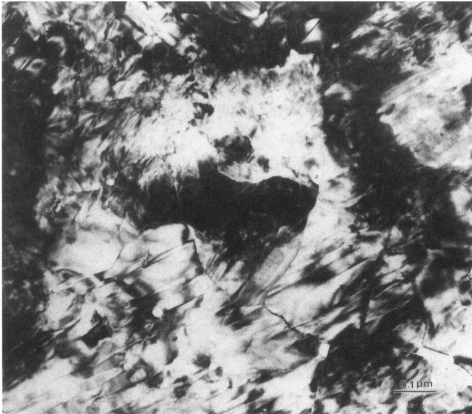
FIG. 4. A typical plan view micrograph of Y-Ba-Cu-O on MgO showing different grain sizes.
