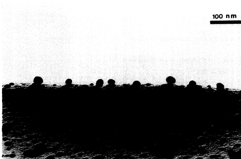
FIG. 1. Electron micrographs of Ag aggregates on a bent substrate of amorphous carbon ( a-C ). T = 20^\circ\text{C} , deposition rate = 0.1 \text{ pm s}^{-1} .
