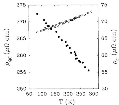
FIG. 1. Anisotropic resistivity and its  $T$  dependence of a thermodynamically stable  $\text{Al}_{62}\text{Si}_3\text{Cu}_{20}\text{Co}_{15}$  2D quasicrystal.
