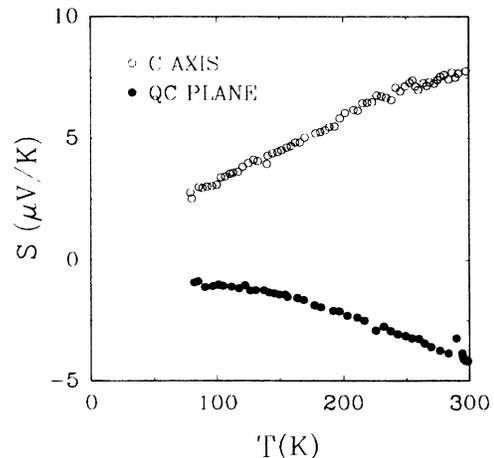
FIG. 4. Anisotropic thermopower of the  $\text{Al}_{62}\text{Si}_3\text{Cu}_{20}\text{Co}_{15}$  2D quasicrystal.
