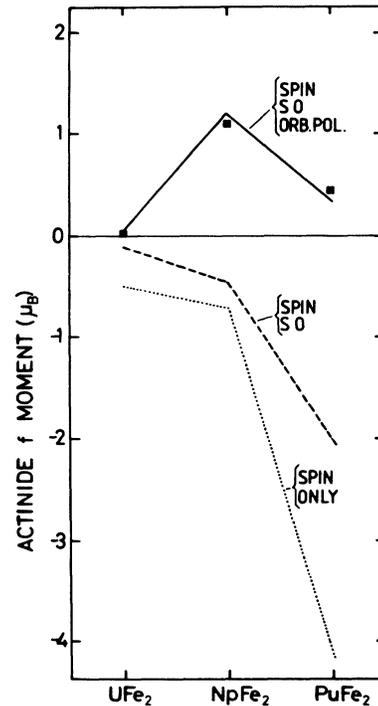
FIG. 5. Calculated (lines) and experimental (squares)  $5f$  moments for UFe<sub>2</sub>, NpFe<sub>2</sub>, and PuFe<sub>2</sub>. The magnetization of Fe is in the positive direction.
