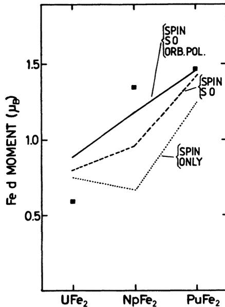
FIG. 6. Calculated (lines) and experimental (squares) 3d moments for  $\text{UFe}_2$ ,  $\text{NpFe}_2$ , and  $\text{PuFe}_2$ .
