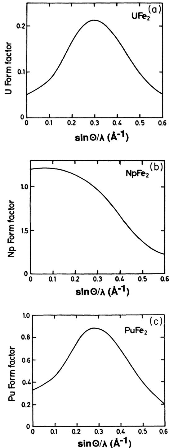
FIG. 7. (a) Magnetic form factor times the magnetic moment for U in  $\text{UFe}_2$ . (b) Magnetic form factor times the magnetic moment for Np in  $\text{NpFe}_2$ . (c) Magnetic form factor times the magnetic moment for Pu in  $\text{PuFe}_2$ .
