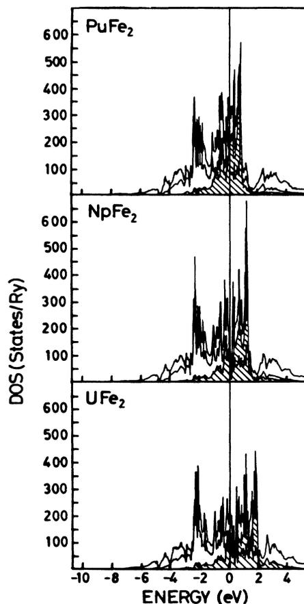
FIG. 1. Calculated DOS for  $\text{UFe}_2$ ,  $\text{NpFe}_2$ , and  $\text{PuFe}_2$ . The upper curve in each panel is the total DOS. The lower curves in each panel are the Fe  $d$  and U  $f$  partial DOS. The area below the U  $f$  DOS is dashed.
