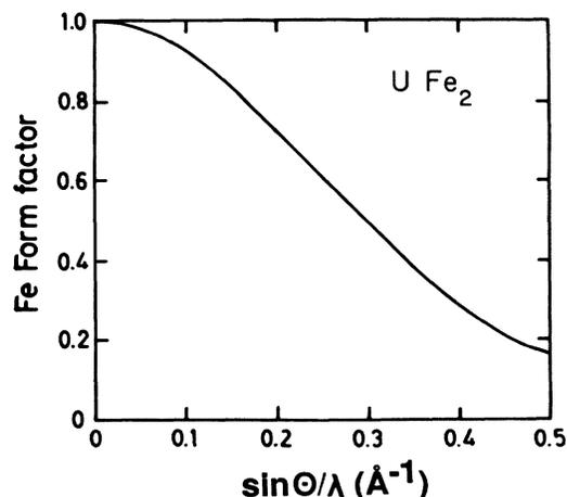
FIG. 8. Magnetic form factor for Fe in  $\text{UFe}_2$ .
