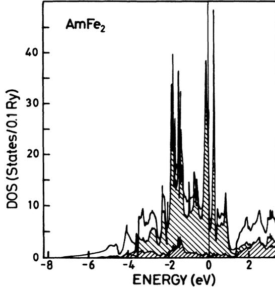
FIG. 2. Calculated DOS for  $\text{AmFe}_2$ . The upper curve is the total DOS. The Fe  $d$  partial DOS is dashed from left to right and the Am  $d$  partial DOS is dashed from right to left. In these calculations the  $5f$  electrons are considered as core electrons.
