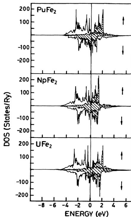
FIG. 4.  $3d$  and  $5f$  partial DOS for  $\text{UFe}_2$ ,  $\text{NpFe}_2$ , and  $\text{PuFe}_2$  from a spin-polarized calculation. The  $5f$  DOS is dashed from left to right and the arrows indicate the spin-up and spin-down DOS.
