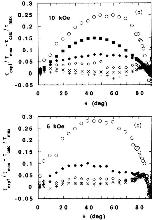
FIG. 4. The differences between the experimental and calculated normalized torques: (a) 10-kOe field:  $\circ$ , 98 K;  $\blacklozenge$ , 96 K;  $\diamond$ , 94 K;  $\times$ , 92 K;  $+$ , 90 K. Also shown as  $\blacksquare$  is the function  $0.15 \sin(2\theta)$ . (b) 6-kOe field:  $\circ$ , 98 K;  $\blacklozenge$ , 96 K;  $\diamond$ , 94 K;  $\times$ , 92 K; and  $+$ , 90 K.
