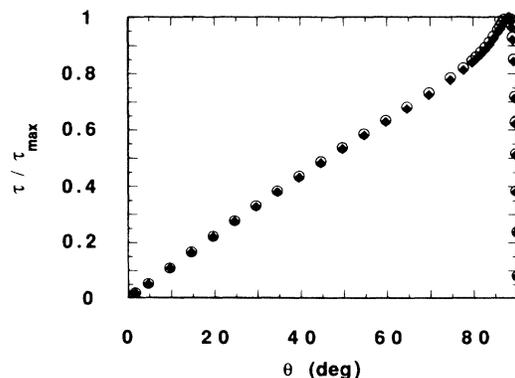
FIG. 3. The normalized torque measured at 90 K in a 10-kOe field at various angles with respect to the  $c$  axis of a  $Tl_2Ba_2CaCu_2O_x$  film ( $\blacklozenge$ ). The predictions of Eq. (1) for  $\gamma = 94$ ,  $\eta H_{c2\parallel}/H = 240$ , and a Gaussian distribution (HWHM =  $0.3^\circ$ ) of  $c$ -axis orientations are shown as  $\circ$ .
