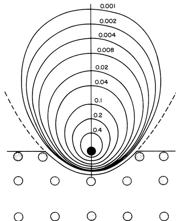
FIG. 1. The geometry of the surface vacancy and the contours of probability density of electron of the half-confined hydrogen atom in ground state in the vacancy ( $v_1=1, v_2=0, m=0$ ). The shape of the potential wall of repulsion is approximately represented by a paraboloid of revolution.  $\xi_0$  is approximately equal to the nearest-neighbor distance of the solid. ●, the nucleus of the impurity-hydrogen atom; ○, the host atom.
