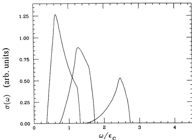
FIG. 4. Diagram representing contribution to intragap infrared absorption at three different values of the hole concentration,  $\delta$ . Frequency is in units of  $\epsilon_c = 4e^2/\epsilon_\infty a_0$ .
