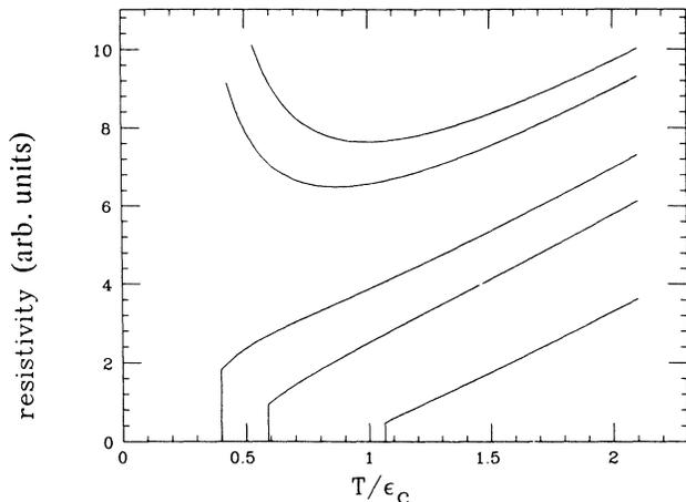
FIG. 5. Resistivity vs temperature for a variety of values of  $\delta$  from Eqs. (49) and (50). [Upper curves:  $(\delta/\delta_c - 1) = -0.01, -0.001$ ; lower curves: 0.3, 0.5, 1.0]. Temperature is in units of  $\epsilon_c$ .
