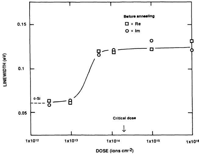
FIG. 2. The linewidth (HWHM) of the  $\frac{3}{2}$ th-derivative spectra. There is an abrupt increase at a dose of about  $3 \times 10^{13}$  ions  $\text{cm}^{-2}$ . The critical dose measured previously ( $2 \times 10^{14}$  ions  $\text{cm}^{-2}$ ) is also indicated (arrow).
