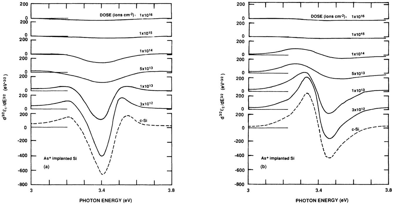
FIG. 1. The  $\frac{3}{2}$ -th-derivative spectra in the  $E_1$  region for  $c$ -Si (dashed lines) and for 150-keV  $\text{As}^+$ -implanted Si at doses from  $3 \times 10^{12}$  to  $1 \times 10^{16}$  ions  $\text{cm}^{-2}$  (solid lines), calculated from the dielectric functions using Eq. (1b). (a) Real parts and (b) imaginary parts.
