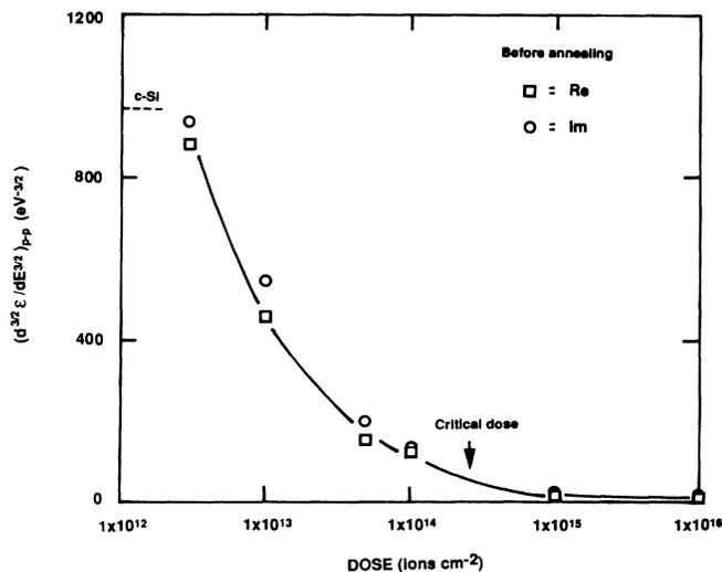
FIG. 3. The peak-to-peak heights of the  $\frac{3}{2}$ th-derivative spectra, drastically decreasing with crystal damage in the implanted region.
