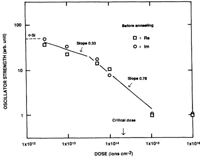
FIG. 4. Oscillator strength vs total dose, found to vary approximately with  $\Phi^{-\beta}$  (solid lines) where initially  $\beta \approx 0.33$ , followed by a transfer to 0.78 at a dose of  $3 \times 10^{13}$  ions  $\text{cm}^{-2}$ ;  $\Phi$  is the dose before saturation.
