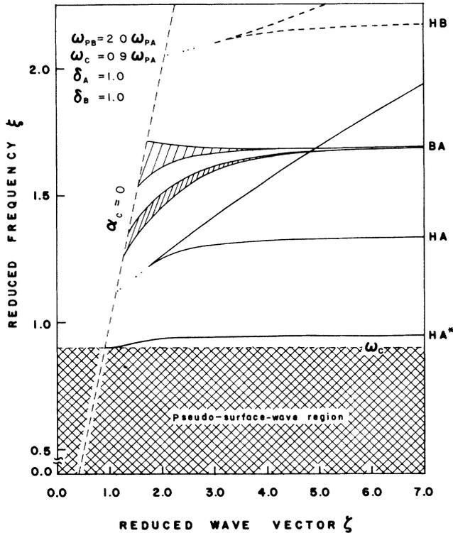
FIG. 7. Dispersion curves for the surface polaritons of the truncated superlattice and the allowed bulk bands (cross-hatched regions) of the infinite superlattice in the presence of a magnetic field, with  $\omega_c = 0.9\omega_{pA}$  and  $\delta_B = \delta_A$ .
