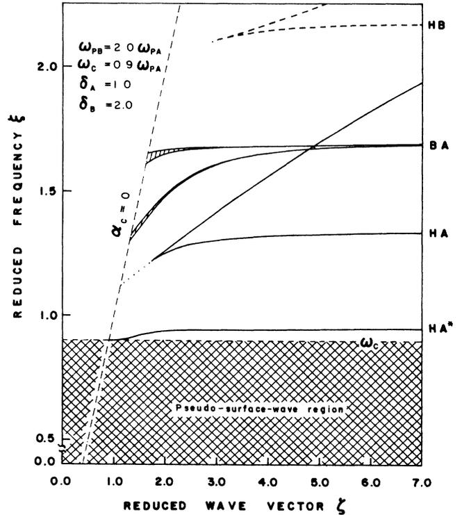
FIG. 10. Dispersion curves for the surface polaritons of the truncated superlattice and the allowed bulk bands (cross-hatched regions) of the infinite superlattice in the presence of a magnetic field, with  $\omega_c = 0.9\omega_{pA}$  and  $\delta_B = 2.0\delta_A$ .
