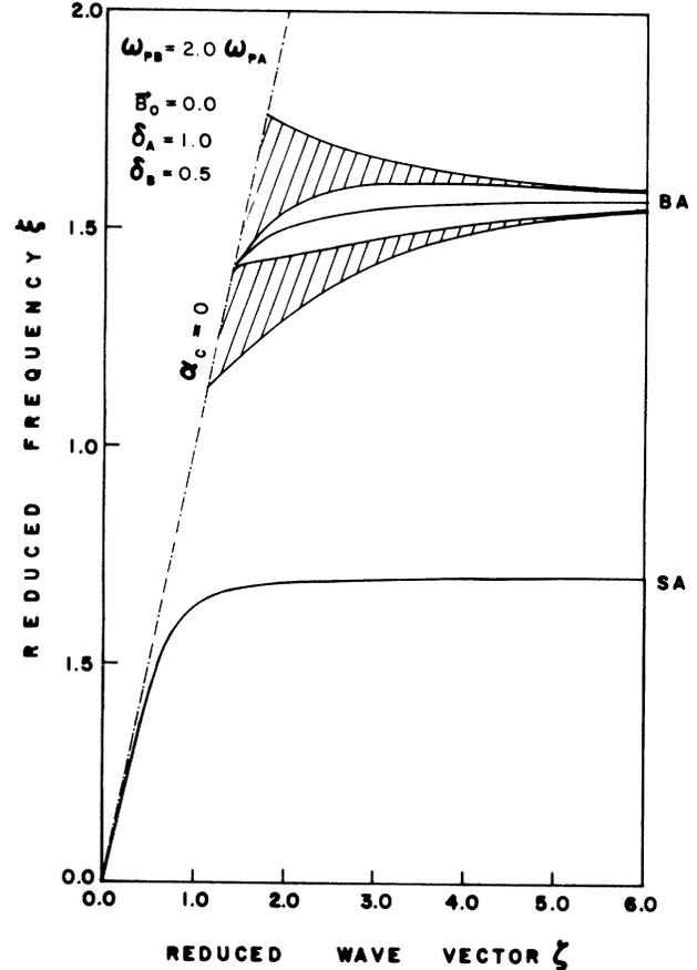
FIG. 2. Dispersion curves for the surface polaritons of the truncated superlattice and the allowed bulk bands (cross-hatched regions) of the infinite superlattice in the absence of a magnetic field, with  $\delta_B = 0.5\delta_A$ . The parameters used are listed in the figure;  $\alpha_c = 0$  is the light line. The letters BA and SA refer to the bulk and surface asymptotic limits.
