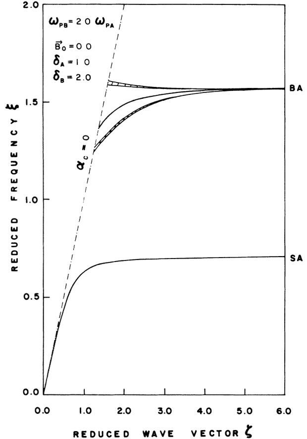
FIG. 8. Dispersion curves for the surface polaritons of the truncated superlattice and the allowed bulk bands (cross-hatched regions) of the infinite superlattice in the absence of a magnetic field,  $\delta_B = 2.0\delta_A$ .
