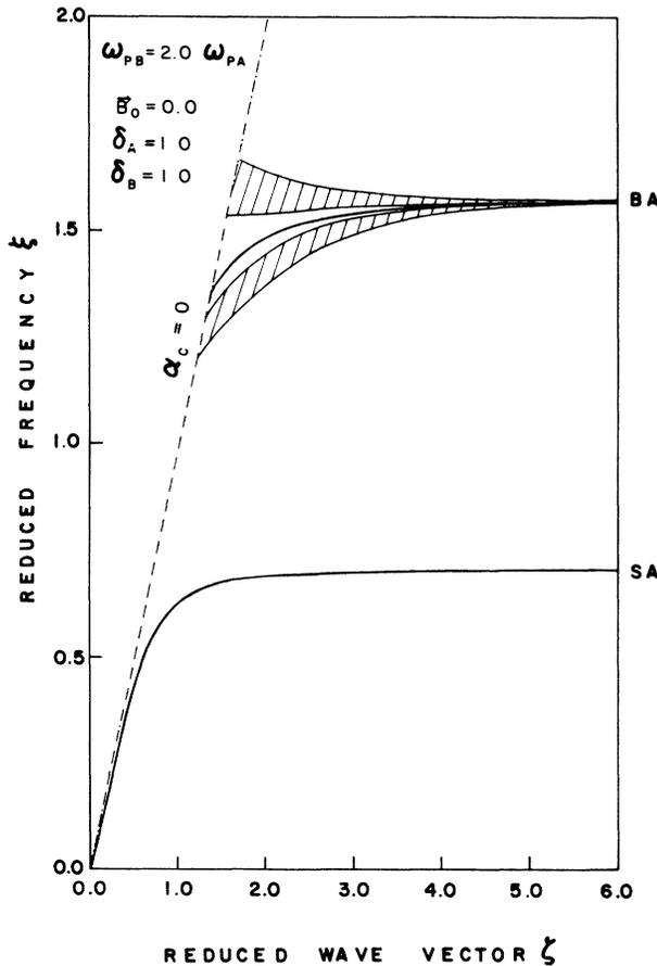
FIG. 5. Dispersion curves for the surface polaritons of the truncated superlattice and the allowed bulk bands (cross-hatched regions) of the infinite superlattice in the absence of a magnetic field, with  $\delta_B = \delta_A$ .
