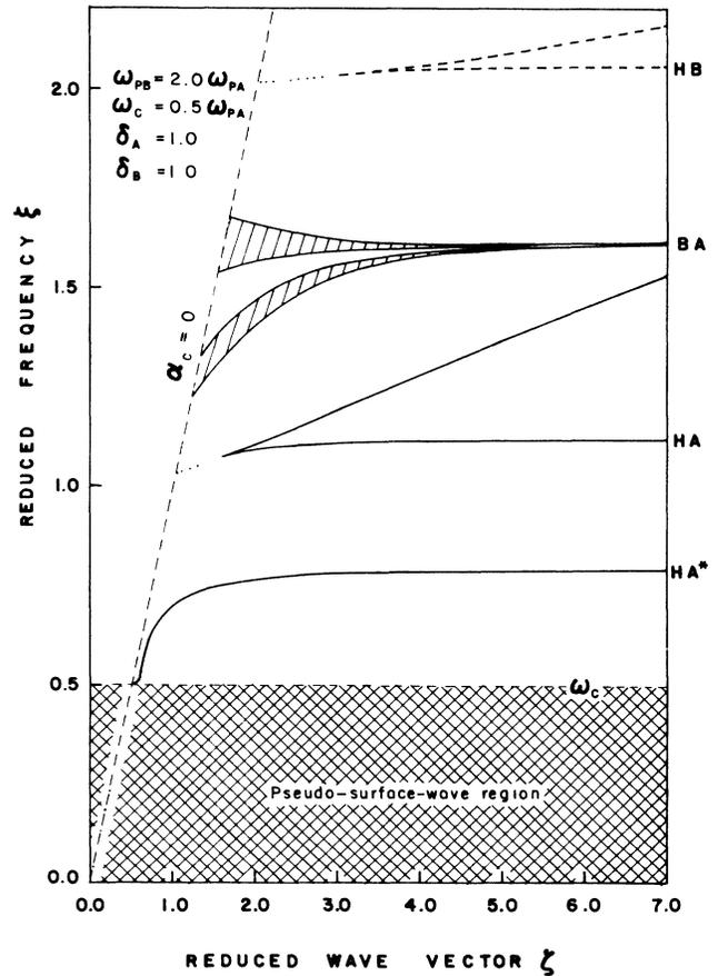
FIG. 6. Dispersion curves for the surface polaritons of the truncated superlattice and the allowed bulk bands (cross-hatched regions) of the infinite superlattice in the presence of a magnetic field, with  $\omega_c = 0.5\omega_{pA}$  and  $\delta_B = \delta_A$ .
