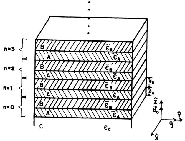
FIG. 1. Schematics of a periodic heterostructure consisting of two different types of metallic slab.
