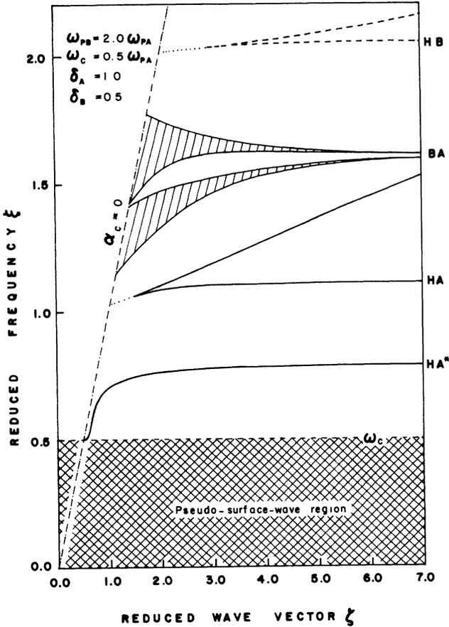
FIG. 3. Dispersion curves for the surface polaritons of the truncated superlattice and the allowed bulk bands (cross-hatched regions) of the infinite superlattice in the presence of a magnetic field, with  $\omega_c = 0.5\omega_{pA}$  and  $\delta_B = 0.5\delta_A$ . The letters  $HA^*$ ,  $HA$ , and  $HB$  refer, respectively, to the asymptotic limits  $\omega_{HA}/\sqrt{2}$ ,  $\omega_{HA}$ , and  $\omega_{HB}$ . The letters  $BA$  stand for the asymptotic limit approached by the bulk bands.
