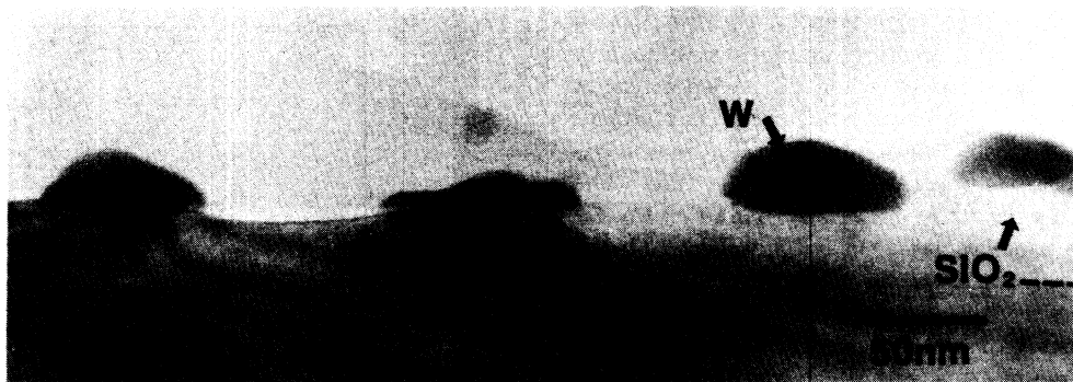
FIG. 3. High-resolution cross-sectional TEM photograph of a 40-Å-thick tungsten layer evaporated on 200 Å of thermal oxide. The sample was vacuum annealed to 1000 °C for 10 min.
