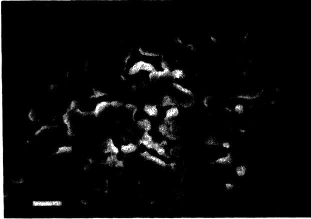
FIG. 1. SEM photograph showing the grain structure and voids present in \text{YBa}_2\text{Cu}_{2.95}\text{Fe}_{0.05}\text{O}_{7-\delta} . The scale bar marks 5 \mu\text{m} .
