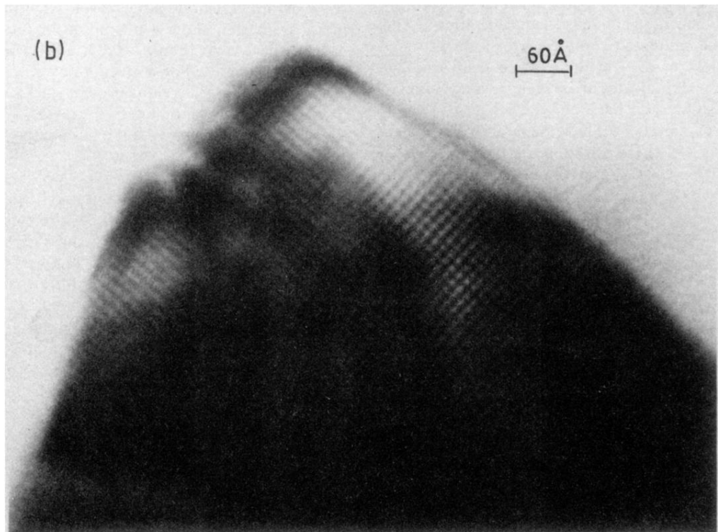
FIG. 4. Typical electron diffraction pattern (a) and lattice image (b) obtained for the x=1.2 sample along the [001] direction showing (5 \times) a \text{K}_2\text{NiF}_4 superlattice and \sim 18 \text{ \AA} fringes.
