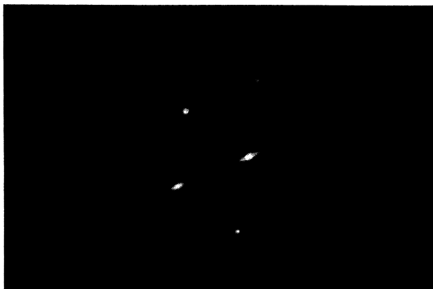
FIG. 4. LEED pattern for a vicinal Si(111) surface misoriented by 6° toward [2\bar{1}\bar{1}] at 360°C. Incident energy = 48 eV. Incident angle = 10° with respect to [111] . Reflection positions and scale as in Fig. 2.
