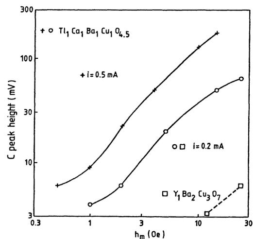
FIG. 3. Modulation amplitude dependence of the peak height of derivative microwave signal from  $Tl_1Ca_1Ba_1Cu_1O_{4.5}$  and from  $Y_1Ba_2Cu_3O_7$  by two microwave intensities ( $i = 0.5$  and  $0.2$  mA).
