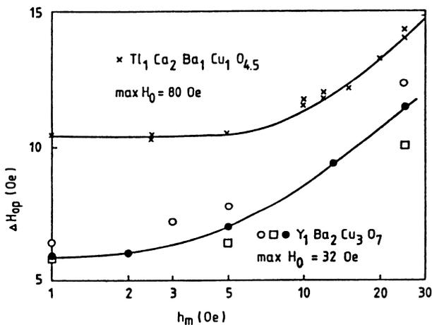
FIG. 5.  $\Delta H_{op}$  half linewidth (the field where the peak of derivative signal appears) vs modulation amplitude for  $Tl_1Ca_1Ba_1Cu_1O_{4.5}$  and for three different Y based samples.
