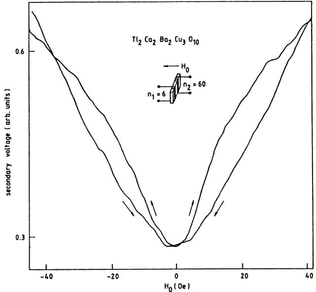
FIG. 12. The secondary voltage vs applied dc magnetic field recorded with phase-lock technique by the superconductor  $Tl_2Ca_2Ba_2Cu_3O_{10}$  core transformer. For both scanning directions the minimum appears at  $H_0=0$  (birdlike shape).
