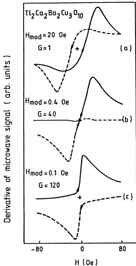
FIG. 4. Derivative of microwave signal from  $Tl_2Ca_2Ba_2Cu_3O_{10}$  for different modulation amplitude: (a)  $h_m = 20$  Oe receiver relative gain  $G = 1$ ; (b)  $h_m = 0.4$  Oe,  $G = 40$  and (c)  $h_m = 0.1$  Oe,  $G = 120$ .
