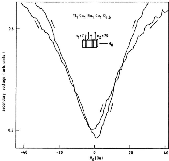
FIG. 11. Secondary voltage vs applied dc magnetic field recorded after phase-sensitive detection for the superconductor  $Tl_1Ca_1Ba_1Cu_1O_{4.5}$  core transformer.
