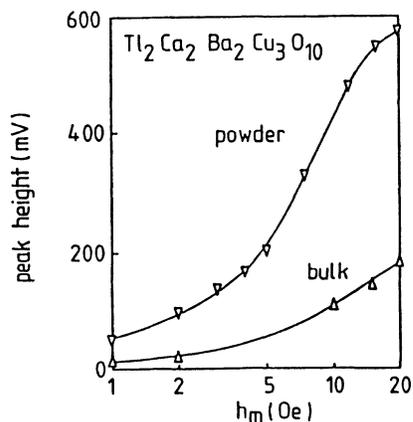
FIG. 15. Magnetic field dependence of microwave derivative signals peak height in bulk ceramic ( $\Delta$ ) and in powder ( $\nabla$ )  $\text{Tl}_2\text{Ca}_2\text{Ba}_2\text{Cu}_3\text{O}_{10}$ .
