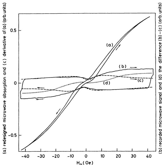
FIG. 9. Magnetic field dependence of (a) the redesigned microwave absorption signal, (b) the recorded derivative signal obtained with weak modulation ( $h_m = 0.01$  Oe) and phase-sensitive detection, (c) the derivative of (a) obtained by graphical differentiation, and (d) the difference between (b) and (c).
