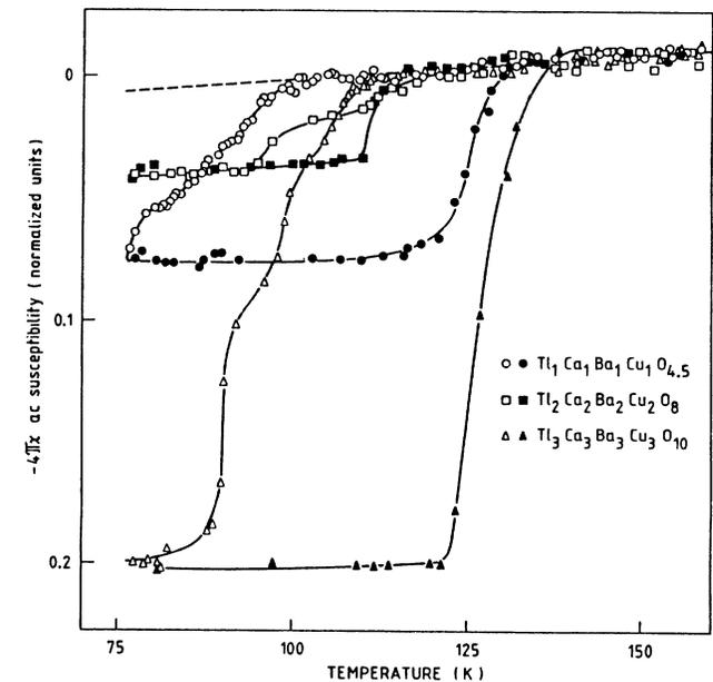
FIG. 13. Temperature dependence of the ac susceptibility in three Tl based compounds. Open symbols indicate decreasing solid symbols increasing temperatures. The magnetic field exclusion starts at 100 K ( $\circ$ ), 120 K ( $\square$ ), and 111 K ( $\triangle$ ).
