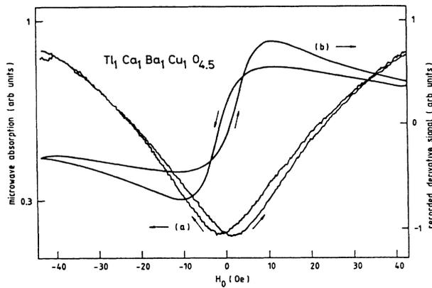
FIG. 8. Magnetic field dependence of microwave absorption signal (a) and the field derivative of microwave signal obtained with modulation ( $h_m = 5$  Oe) and phase sensitive detection (b) in  $\text{Tl}_1\text{Ca}_1\text{Ba}_1\text{Cu}_1\text{O}_{4.5}$ .
