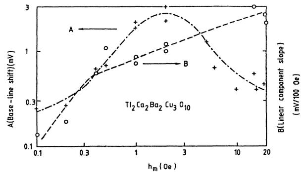
FIG. 2. Modulation amplitude dependence of the base-line shift (*A*) and mostly linear (*B*) component of the derivative signal from  $Tl_2Ca_2Ba_2Cu_3O_{10}$ . Lines are guides for the eye.
