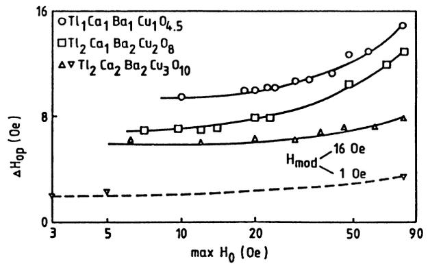
FIG. 6. The  $\Delta H_{op}$  half linewidth vs scan field amplitude (max  $H_0$ ) observed in three Tl compounds, for  $h_m = 16$  Oe and in  $Tl_2Ca_2Ba_2Cu_3O_{10}$  for  $h_m = 1$  Oe too.
