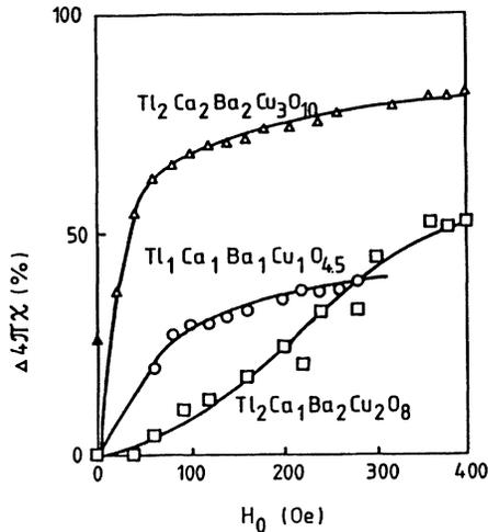
FIG. 14. Magnetic field strength dependence of the ac susceptibility at 77 K in three Tl based compounds. The solid triangle represents the remanent susceptibility modification for one of the samples. The comparison of Figs. 14, 13, and 7 indicates a connection between the field dependence of ac susceptibility and field amplitude dependence of microwave signal.
