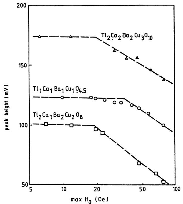
FIG. 7. The peak height vs scanning dc field amplitude (max  $H_0$ ) for three Tl compounds at  $h_m = 16$  Oe. The straight lines are guides for the eye.
