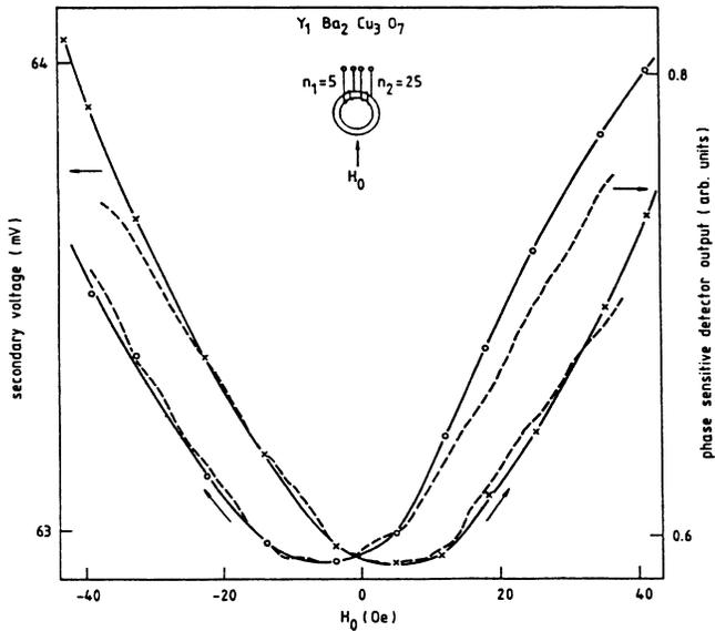
FIG. 10. Magnetic field dependence of secondary voltage of the  $Y_1Ba_2Cu_3O_7$  superconductor core transformer measured with DMM and recorded after phase-sensitive detection. Both methods give the same result. Two, about  $H_0=0$  symmetrically placed minima appear.
