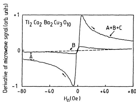
FIG. 1. Representative microwave signal related to field derivative of absorption in  $Tl_2Ca_2Ba_2Cu_3O_{10}$  using  $h_m = 1$  Oe modulation amplitude, at  $T = 77$  K, by forward and backward field scan.
