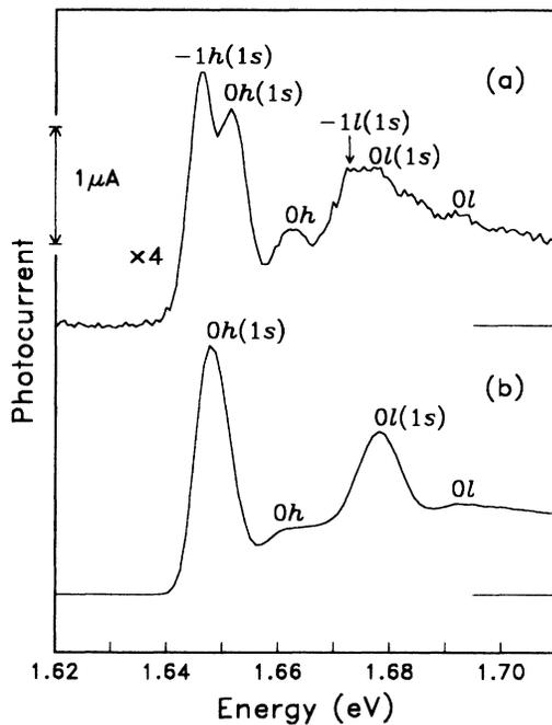
FIG. 1. Photocurrent spectra of a (40 Å/40 Å) GaAs/Ga<sub>0.65</sub>Al<sub>0.35</sub>As superlattice at 5 K for two representative values of the electric field applied normal to the layers. (a) 10 kV/cm and (b) 40 kV/cm.
