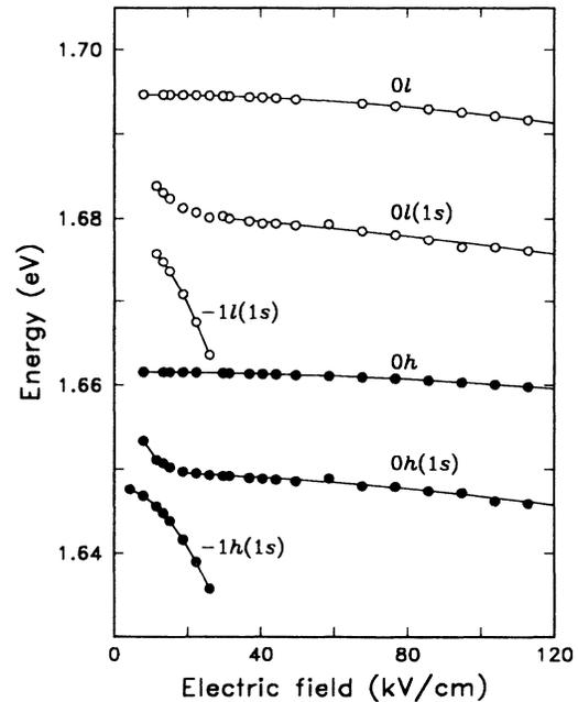
FIG. 2. Electric-field dependence of the transition energies for heavy holes (solid circles) and for light holes (open circles) obtained from photocurrent spectra. The separation between  $0h(1s)$  [ $0l(1s)$ ] and  $0h$  [ $0l$ ] peaks gives the binding energy for heavy- and (light-) hole excitons.
