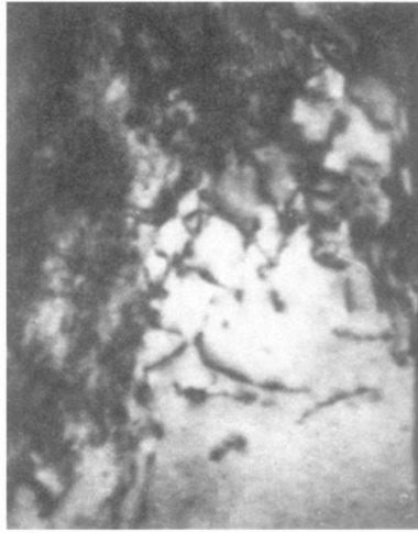
FIG. 10. Electron-microscope image (magnification: 1.35 \times 10^5 ) for the specimen of the Ni alloy with oxygen.
