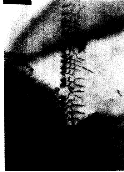
FIG. 12. The typical diffraction contrast image (magnification: 2.8 \times 10^4 ) for the specimen of a Ni-Fe-based alloy with oxygen.
