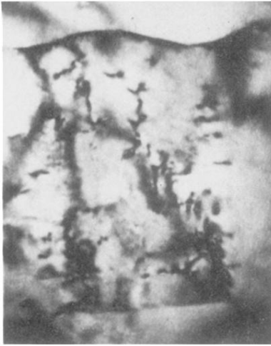
FIG. 9. The image of an electron microscope (magnification: 1.35 \times 10^5 ) for the specimen of a Ni alloy without oxygen.
