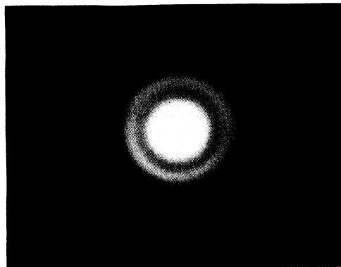
FIG. 4. TEM diffraction pattern of sample 2.
