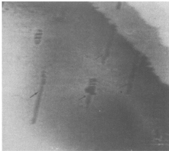
FIG. 7. 120 \times 90\text{-}\text{\AA}^2 image at +1 V. The O row appears as a trough due to the O-chemisorbed W tip.
