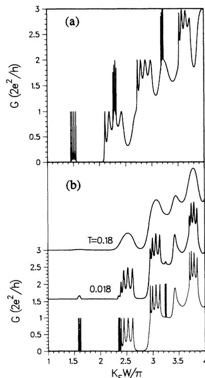
FIG. 4. Conductance for five-period superlattices with (a)  $V_{sl} = 3$ , and (b)  $V_{sl} = 5$ . Temperature effects are shown to smooth out only the sharpest features.  $T = 0.018 \simeq 120$  mK in typical system (see text).
