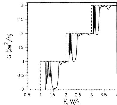
FIG. 2. Conductance for 1DSL with five periods vs Fermi wave number (solid line). Dashed line, conductance steps in ideal unmodulated constriction. Notice strong resonances and subband onsets moved upwards by superlattice effects.
