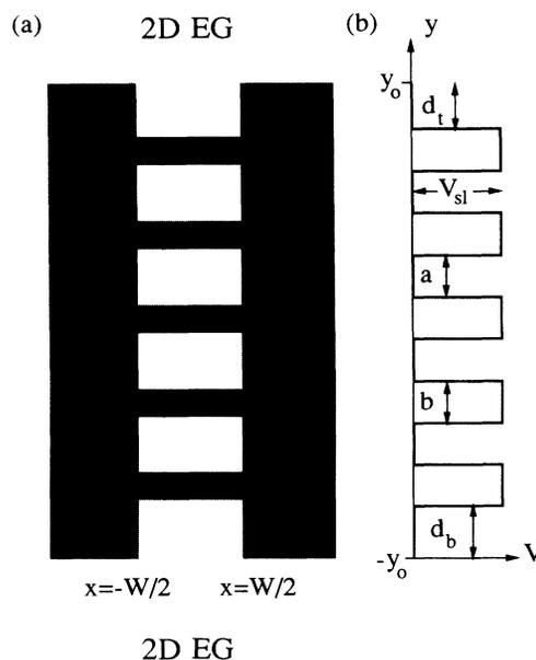
FIG. 1. Constriction extends along  $y$  axis, width  $W$ . Shaded areas represent negatively biased gate.
