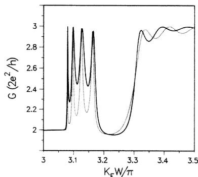
FIG. 3. Conductance  $G_{IB}$  (solid line) and  $G$  (dotted) for third plateau in system of Fig. 2. Sharper superlattice features in  $G$  are due to longitudinal resonance effects.
