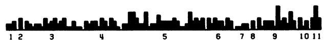
FIG. 1. An example of patterns formed on a segment divided into 100 unit cells. There are 11 clusters numbered from 1 to 11. The area, surface, and bottom length of clusters are denoted, by A , L , and B , respectively. For example, A , L , and B of number 1 are equal to 7, 9, and 3.
