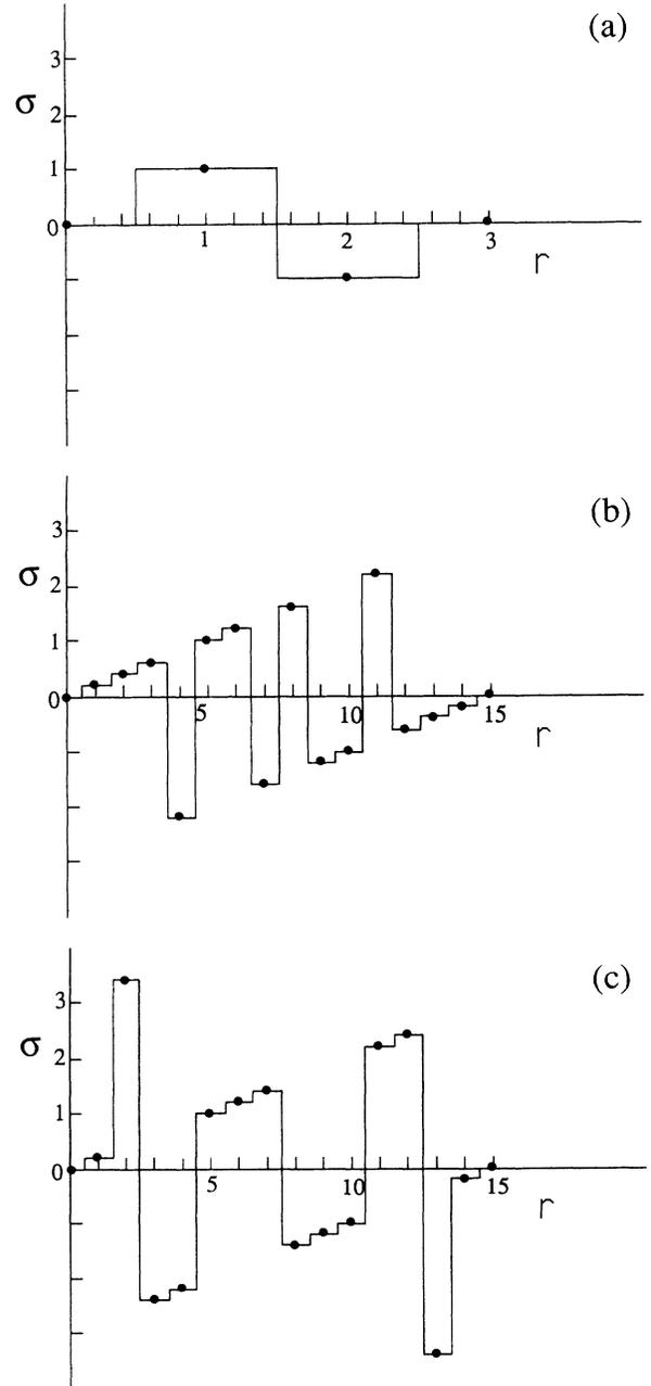
FIG. 2. Hall conductivity  $\sigma$  in a plane (a) when the field and the  $c$  direction are colinear; (b) when the direction  $c$  is tilted ( $p'/q' = \frac{1}{5}$ ); (c) when  $p'/q' = \frac{2}{5}$ . The lines are guides for the eyes: The Hall conductivity is only computed in the gaps. The conductivity is expressed in units of  $e^2/h$ .
