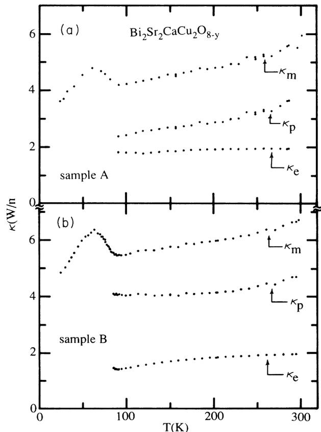
FIG. 4. Temperature dependence of measured *ab*-plane thermal conductivity  $\kappa_m$  shown with deduced phonon and electron components ( $\kappa_p$  and  $\kappa_e$ ) for (a) sample A and (b) sample B.
