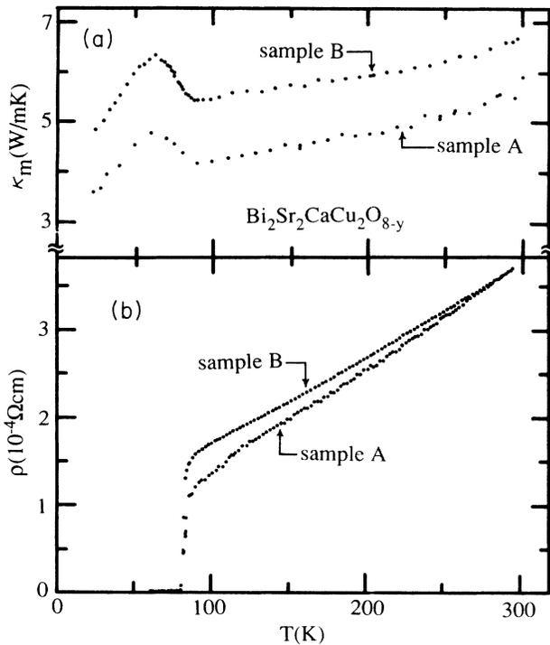
FIG. 1. (a) Measured  $ab$ -plane thermal conductivity vs temperature for two metallic crystals of  $\text{Bi}_2\text{Sr}_2\text{CaCu}_2\text{O}_{8-y}$ . (b)  $ab$ -plane resistivity vs temperature for the same two crystals.
