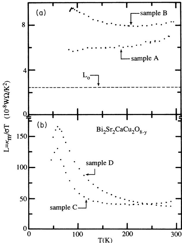
FIG. 3. *ab*-plane Lorenz ratio,  $L = \kappa_m / \sigma T$ , for (a) the two metallic crystals shown in Fig. 1 (the Sommerfeld value,  $L_0 = 2.45 \times 10^{-8} \text{ W}\Omega/\text{K}^2$ , is included for comparison) and (b) the two nonmetallic, oxygen-deficient crystals shown in Fig. 2.
