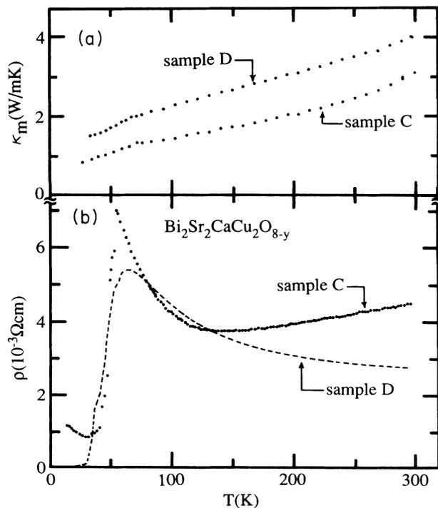
FIG. 2. (a) Measured  $ab$ -plane thermal conductivity for two nonmetallic oxygen-deficient crystals of  $\text{Bi}_2\text{Sr}_2\text{CaCu}_2\text{O}_{8-y}$ . (b)  $ab$ -plane resistivity vs temperature for the same two crystals.
