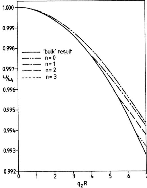
FIG. 4. Interface mode dispersion curves for a 50-Å wire. The bold solid curve corresponds to the "bulk" result (17). Note that the various interface modes (here corresponding to  $n=0,1,2,3$ ) emerge from this curve.
