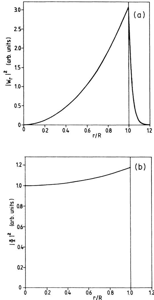
FIG. 5. Variation in the radial component of the displacement (a) and its associated potential (b) for the  $n=0$  interface mode of a 50-Å wire ( $q_z R = 2.0$ ). The units are not related to those of Fig. 3.
