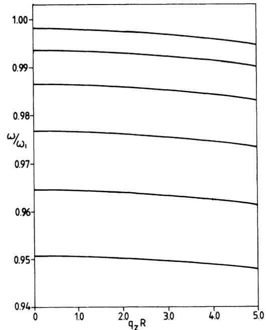
FIG. 2. Dispersion of the allowed  $n=0$  guided modes for a 50-Å wire radius.
