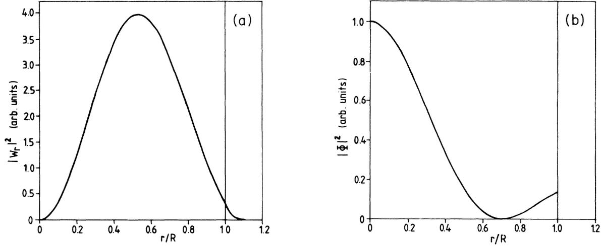
FIG. 3. (a) Variation in the radial component of the displacement and (b) its associated potential for the highest frequency  $n=0$  guided mode of a 50-Å wire ( $q_2 R = 2.0$ ).
