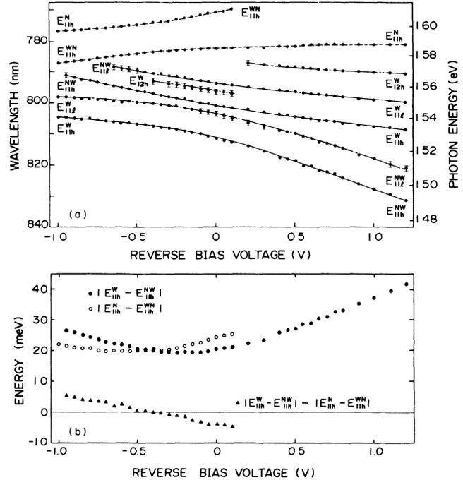
FIG. 3. (a) Absorption peak wavelengths (energies) as a function of bias voltage  $V_{ex}$ . The observed optical transitions are divided into four pairs. (b) The  $V_{ex}$  dependence of the separation energies between the paired optical transitions associated with the  $h_1^W$  heavy-hole level,  $|E_{11h}^W - E_{11h}^{NW}|$ ,  $|E_{11h}^N - E_{11h}^{WN}|$ , and their differences,  $|E_{11h}^W - E_{11h}^{NW}| - |E_{11h}^N - E_{11h}^{WN}|$ .
