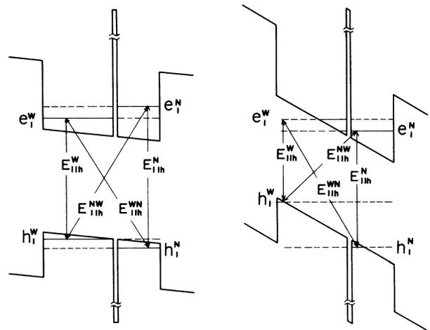
FIG. 1. Schematically illustrated energy-band diagrams of an asymmetric double-quantum-well structure in two different electric fields. Pay attention to the relative positions of  $e_1^W$  and  $e_1^N$  quantized levels. For clarity, the light-hole levels and the higher-lying levels are eliminated. Some optical transitions are inserted.
