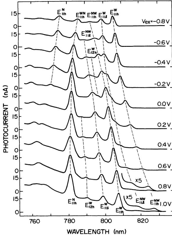
FIG. 2. Photocurrent spectra of an asymmetric coupled-quantum-well structure at different bias voltages. Four pairs of 100- and 60-Å-thick GaAs wells, separated by 4-Å-thick AlAs barriers, are embedded in the intrinsic region sandwiched between *p*- and *n*-type AlAs-GaAs superlattices. Measurements were made at 77 K. Reverse bias is positive.
