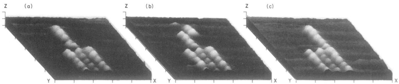
FIG. 3. STM images over an area of  $50 \times 50 \text{ \AA}^2$ , recorded with  $V_t \approx 0.4 \text{ V}$  and  $I_t \approx 1.0 \text{ nA}$ . The three images, formed by line scans in  $x$ , are taken at 3-sec intervals. The dynamical movement of a single Cu-O chain segment between the three chains is directly visible.
