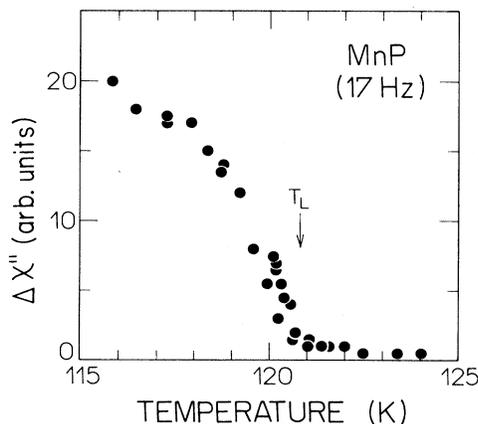
FIG. 2. Height of the peak in  $\chi''$  at the transitions from the ferromagnetic phase as a function of  $T$  for the determination of  $T_L$ .
