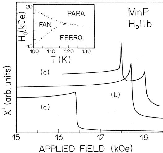
FIG. 1. Traces of the in-phase ac susceptibility vs applied magnetic field at various temperatures: Curve (a),  $T=114.6$  K; curve (b),  $T=121.4$  K; curve (c),  $T=154$  K. The curves are displaced vertically for more clarity. Inset: Phase diagram near  $T_L$ , determined from the susceptibility measurements.
