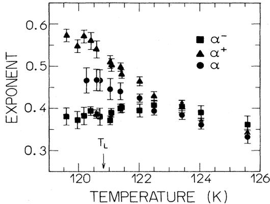
FIG. 4. Values obtained for the critical exponent near  $T_L$ .  $\alpha^-$  and  $\alpha^+$  resulted from the independent fits of the two branches of data.  $\alpha$  is from the fits with the constraints  $\alpha^+ = \alpha^-$  and  $H_c^+ = H_c^-$ .
