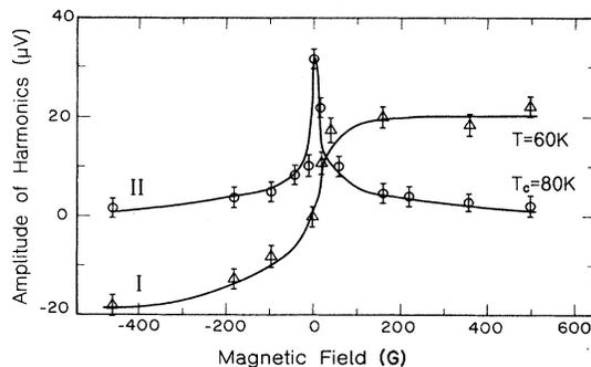
FIG. 5. The dependence of the amplitudes of the first and second harmonics on the magnitude of the dc magnetic field parallel to the film.  $H_1 = 15$  G;  $f = 132$  Hz.
