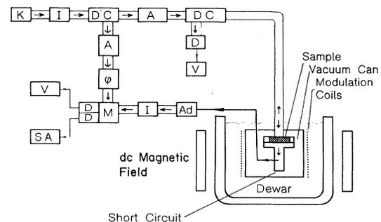
FIG. 1. Schematic description of the experimental system for the determination of the transmission (both magnitude and phase) and reflection. K—Klystron; I—Isolator; DC—directional coupler; A—attenuator; V—digital voltmeter;  $\phi$ —phase shifter; Ad—adapter; M—mixer; SA—spectral analyzer.
