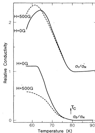
FIG. 6. The temperature dependence of  $\sigma_1$  and  $\sigma_2$  calculated using the data in Fig. 2 and Eqs. (1a) and (1b).
