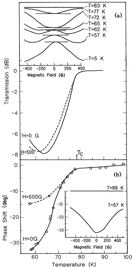
FIG. 2. (a) Transmission amplitude vs temperature at  $H_0=0$  and 500 G. Inset: The transmission vs dc magnetic field at zero field is denoted by horizontal lines. (b) Temperature dependence of the phase shift at  $H_0=0$  and 500 G. Inset: The phase shift vs dc magnetic field in normal and superconducting states.
