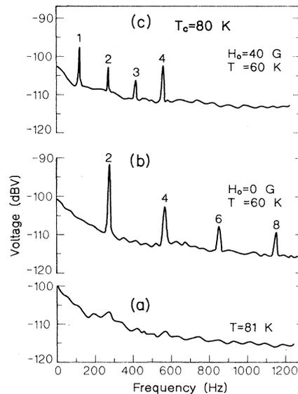
FIG. 3. The low-frequency spectrum of transmitted power through a film ( $T_c=80$  K) in the presence of an ac magnetic field perpendicular to the film. (a) Normal state,  $H_1=15$  G,  $f=132$  Hz,  $T=81$  K. (b) Superconducting state,  $H_1=15$  G,  $f=132$  Hz,  $H_0=40$  G,  $T=60$  K. (c) Superconducting state,  $H_1=15$  G,  $f=132$  Hz,  $H_0=0$  G,  $T=60$  K. Note the even harmonics in (b) but the generation of additional odd harmonics in (c).
