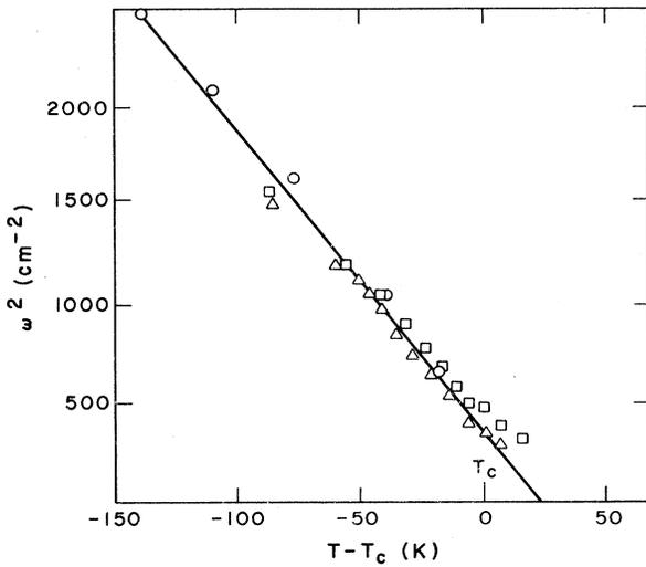
FIG. 3.  $A_g(ZZ, YY, XX)$  soft-mode frequency square vs temperature in  $\text{LaP}_5\text{O}_{14}$ :  $ZZ(\Delta)$ ,  $YY(\square)$  and in  $\text{TbP}_5\text{O}_{14}$ :  $XX(\circ)$ . The solid straight line is identical to the straight line of the low-temperature branch in Fig. 2.
