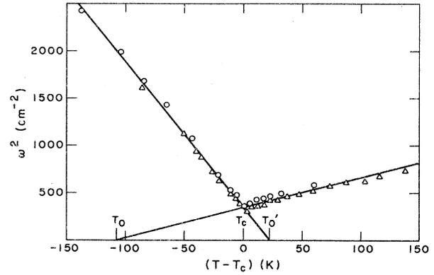
FIG. 2.  $A_g$ - $B_{2g}$ ( $ZX$ ) soft-mode frequency square vs temperature in  $RP_5O_{14}$ . Both  $\text{LaP}_5O_{14}$  ( $\Delta$ ) and  $\text{TbP}_5O_{14}$  ( $\circ$ ) data are included. The least-squares fit give the parameters:  $2B/B' = -4.8$ ;  $1/g = 109^\circ\text{C}$ ;  $1/g' = 23^\circ\text{C}$ .
