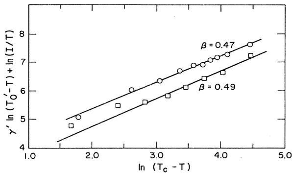
FIG. 7. Double logarithmic plot of ZZ (○) and YY (□) polarizability intensity of  $\text{LaP}_5\text{O}_{14}$ .
