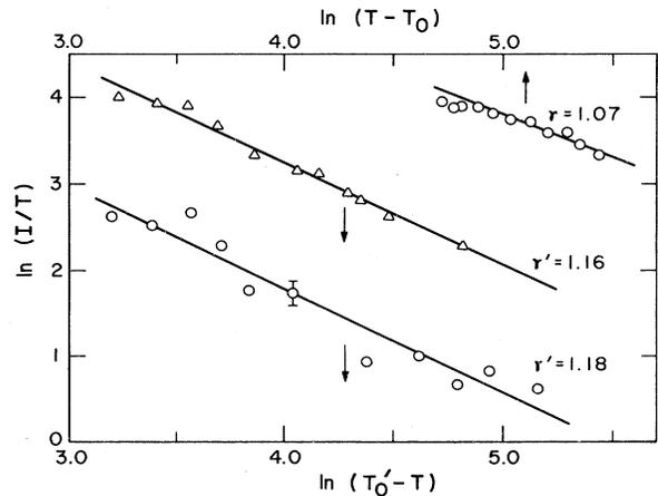
FIG. 6. Double logarithmic plot of  $ZX$  polarizability intensity of  $\text{LaP}_5\text{O}_{14}$  ( $\Delta$ ),  $\text{TbP}_5\text{O}_{14}$  ( $\circ$ ) for  $T < T_c$ , and of  $\text{LaP}_5\text{O}_{14}$  ( $\square$ ) for  $T > T_c$ .
