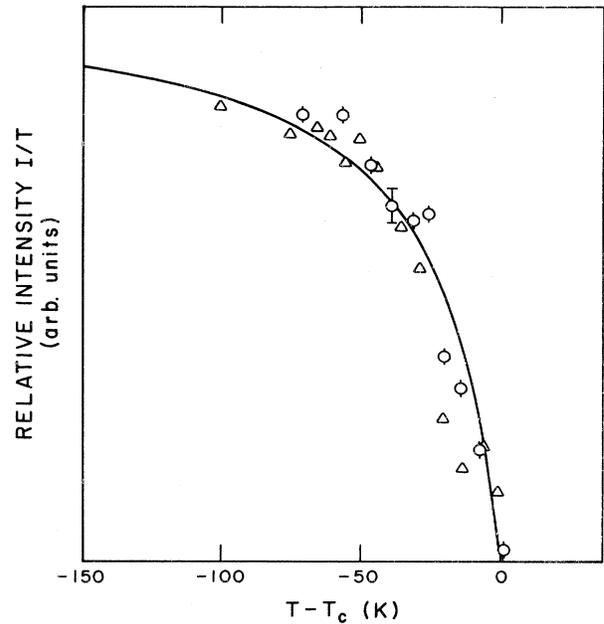
FIG. 5.  $ZZ(\Delta)$ ,  $YY(\square)$  polarizability intensities in  $\text{LaP}_5\text{O}_{14}$ . The solid curve is a fit to the theoretical  $I_2/T$  in Table I for quadratic coupling of  $\eta$  to  $\mathcal{E}$ , with parameters given in the text and in the caption of Fig. 2.
