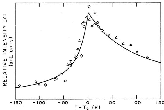
FIG. 4.  $ZX$  polarizability intensities in  $\text{LaP}_5\text{O}_{14}$  ( $\square$ ) and  $\text{TbP}_5\text{O}_{14}$  ( $\circ$ ). The solid curve is a fit to the theoretical  $I_1/T$  described in Table I for linear coupling of  $\eta$  to  $\mathcal{E}$ , with parameters given in the text and in the caption of Fig. 2.
