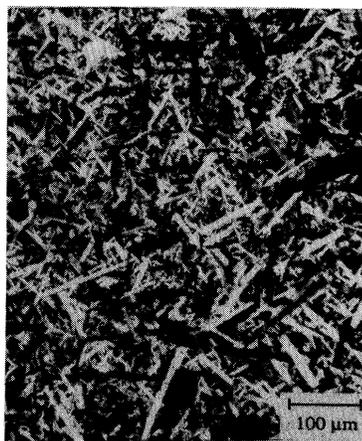
FIG. 2. Micrograph of  $\text{YBa}_2\text{Cu}_3\text{O}_{7-\delta}$  made from material No. 1 taken using polarized light. The bar represents  $100 \mu\text{m}$ .
