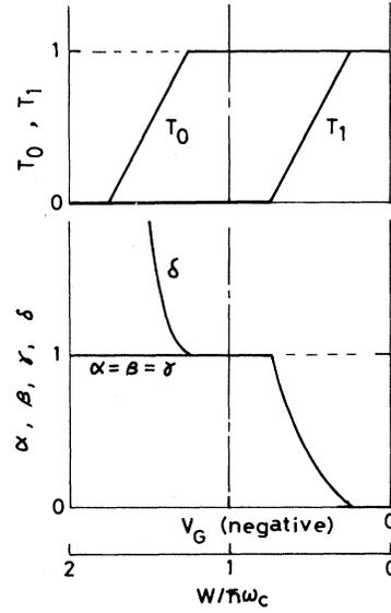
FIG. 3. Characteristics of the disordered contact shown in Fig. 2(b) in the two-channel case. Transmission probabilities  $T_0$  and  $T_1$ , and the parameters  $\alpha$ ,  $\beta$ ,  $\gamma$ , and  $\delta$  are schematically shown as a function of negative gate-bias voltage,  $V_G$ , with respect to the 2D EG.
