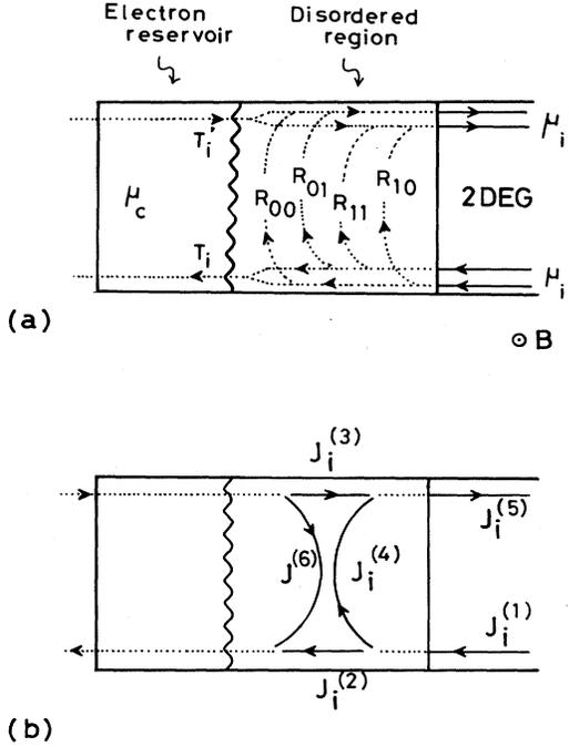
FIG. 1. A schematic representation of a disordered contact, consisting of an electron reservoir and a disordered region. (a) Transmission and reflection probabilities. (b) Characteristic currents relating to the  $i$ th Landau level.
