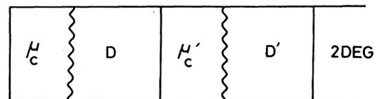
FIG. 4. An example of a generalized disordered contact consisting of two sets of electron reservoirs and disordered regions.
