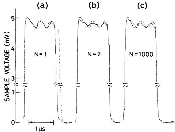
FIG. 6. Comparison between snapshots of the CDW response to the  $N=1$  pulse (solid line) and to a pulse with the old width (dotted line). (b),(c) Comparison between the CDW response to  $N=2$  ( $N=1000$ ) (solid line) and  $N=1$  (dotted line).
