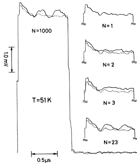
FIG. 7. Sequential responses of the virgin CDW to a train of constant current pulses (solid lines). The response to the initial pulse is shown for comparison by dotted lines.
