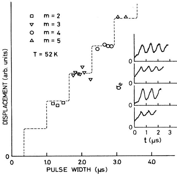
FIG. 2. Displacement of the CDW within a pulsed field as a function of the pulse width (arbitrary unit). The dotted line is a guide for the eye. Inset: Dependence of the extra conductivity due to sliding CDW on the pulse width.
