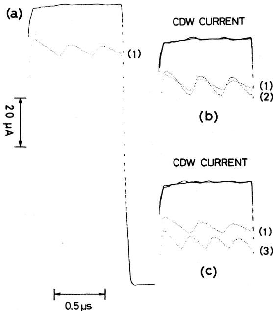
FIG. 3. (a) The total current measured (the solid line) and the single particle current (the dotted line) for the pulsed voltage indicated by (1) in Fig. 1. The difference between them corresponds to CDW current  $J_{\text{CDW}}(t)$ . (b),(c) Comparison between CDW currents for pulsed voltages with different heights shown in Fig. 1.
