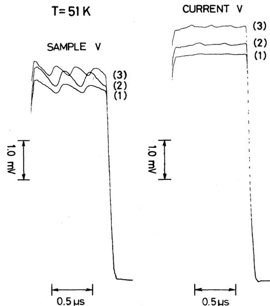
FIG. 1. Pulsed voltages developing across the sample (sample *V*) and across the standard resistor (current *V*) with different pulse heights but the same pulse width. Pulse height increases from (1) to (3). The threshold voltage  $V_T$  of the sample is 3.5 mV at  $T = 51$  K. Value of the standard resistor is 50.7  $\Omega$ .
