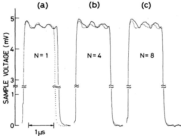
FIG. 5. (a) Comparison between snapshots of the CDW response to  $N=1$  pulse (solid line) and to a pulse with the old width (dotted line). (b),(c) Comparison between the CDW response to  $N=4$  ( $N=8$ ) (solid line) and  $N=1$  (dotted line). The measurements are carried out by using nearly constant current pulse.
