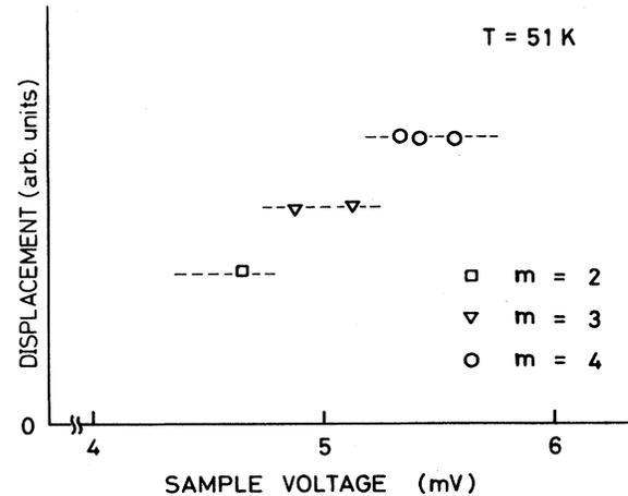
FIG. 4. CDW displacement within a pulse with a given width  $T=0.9 \mu\text{s}$  as a function of the sample voltage averaged over the pulse width (arbitrary unit). The dotted lines are guides for the eye.
