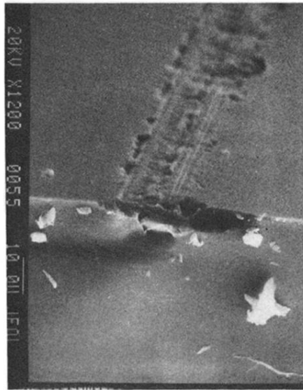
FIG. 5. Scanning electron microscope image of a scribed channel in silicon. Here a wafer was fractured perpendicular to a scratch and the image was taken at an angle of 75^\circ from the normal to the planar surface.
