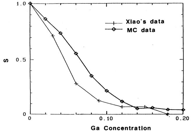
FIG. 9. Oxygen order parameters  $S$  of the  $\text{YBa}_2\text{Cu}_{3-x}\text{M}_x\text{O}_7$  system as a function of the impurity concentration  $x$  at 300 K from Monte Carlo simulations and from data of Xiao *et al.* (Ref. 19).
