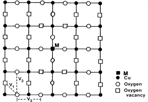
FIG. 8. The structure of the basal plane of the  $\text{YBa}_2\text{Cu}_{3-x}\text{M}_x\text{O}_7$  system with a single impurity  $M$ .
