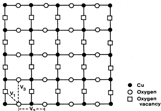
FIG. 1. The ground-state structure of the CuO plane of the  $\text{YBa}_2\text{Cu}_3\text{O}_7$  system.
