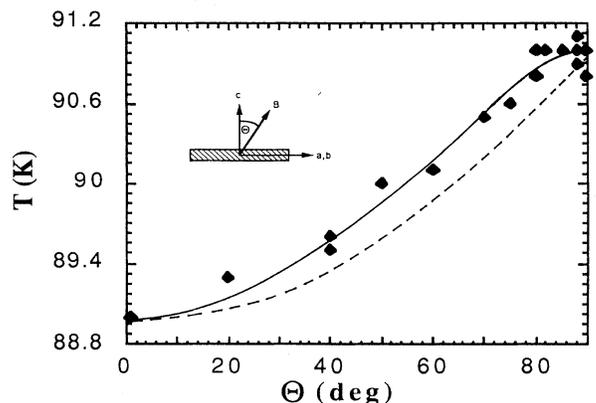
FIG. 4. Angular dependence of  $T_{c2}$ . The solid line is a fit to the anisotropic GL theory with a mass anisotropy of 25. The dashed line is a fit to Tinkham's 2D thin-film model.
