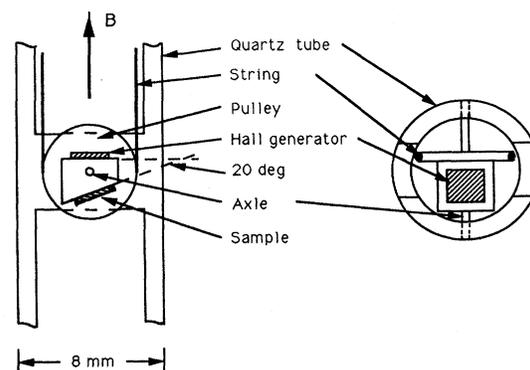
FIG. 1. Design of the sample rotator for dc-magnetization measurements in a SQUID magnetometer.
