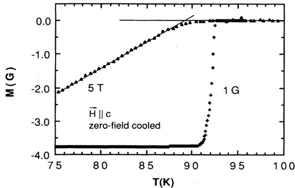
FIG. 2. Zero-field-cooled magnetization curves in fields of 1 G and 5 T perpendicular to the CuO planes. The straight lines indicate the construction of the nucleation temperature  $T_{c2}$ .
