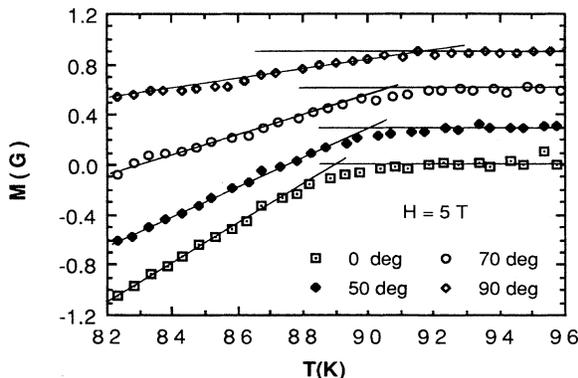
FIG. 3. Temperature dependence of the magnetization in a field of 5 T for different orientations of the  $c$  axis with respect to the field.
