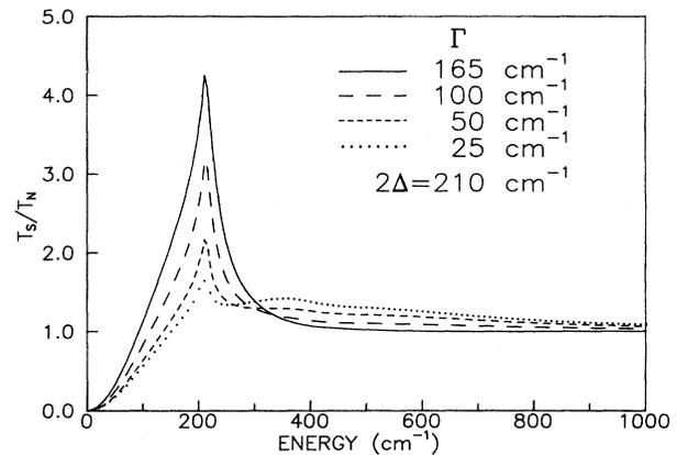
FIG. 2. The ratio of superconducting to normal transmittance for a superconductor in the clean limit ( $\Gamma < 2\Delta$ ). The energy gap was chosen to be  $210 \text{ cm}^{-1}$ . Note that the energy-gap feature disappears in the very clean limit.
