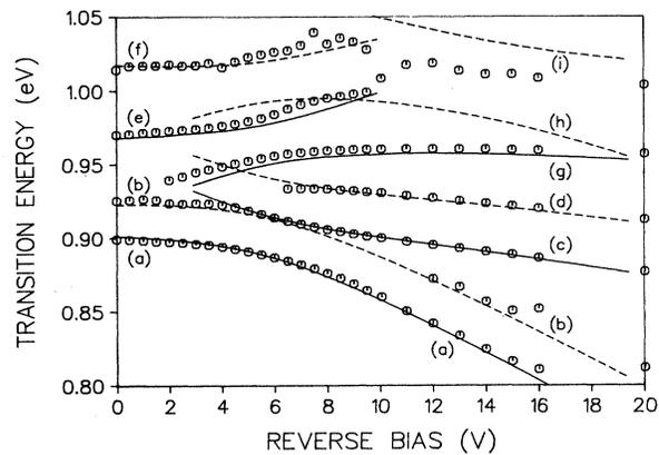
FIG. 5. Comparison of calculated and observed (at 8 K) transition energies for the ACQW structure. Transitions are labeled as in Figs. 2–4. Solid lines indicate heavy-hole transitions and dashed lines are light-hole transitions.
