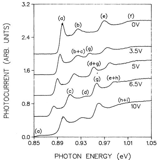
FIG. 4. Low-temperature (8-K) photocurrent spectra of the sample described in Fig. 3. The transitions are labeled as in Figs. 2 and 3, with the addition of (e)  $h_2e_2$ , (f)  $l_2e_2$ , (g)  $h_2e_1$ , (h)  $l_2e_1$ , and (i)  $l_3e_1$ . The spectra are offset vertically for clarity.
