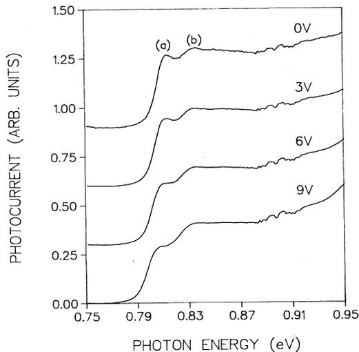
FIG. 2. Room-temperature photocurrent spectra of a sample containing 40 periods of 7.5-nm  $\text{In}_{0.53}\text{Ga}_{0.47}\text{As}$  quantum wells, for several values of reverse bias. Transitions are labeled as follows: (a)  $h_1e_1$  and (b)  $l_1e_1$ . The "noise" in the spectra at about 0.9 eV is due to atmospheric absorptions. The spectra are offset vertically for clarity.
