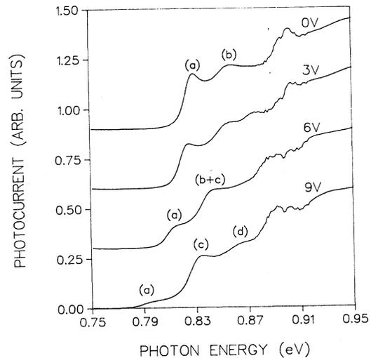
FIG. 3. Room-temperature photocurrent spectra of a sample containing 29 periods of 7.5- and 5.0-nm  $\text{In}_{0.53}\text{Ga}_{0.47}\text{As}$  quantum wells coupled by a 1.6-nm  $\text{In}_{0.52}\text{Al}_{0.48}\text{As}$  barrier, for several values of reverse bias. The transitions are labeled as in Fig. 2, with the addition of (c)  $h_1e_2$  and (d)  $l_1e_2$ . Beyond resonance,  $h_1e_1$  is an interwell transition. The spectra are offset vertically for clarity.
