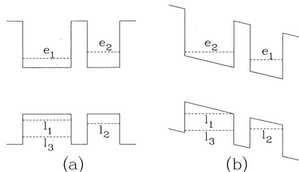
FIG. 1. Energy-band diagram (not to scale) for the asymmetric coupled-quantum-well system for (a) zero field and (b) a field for which the electron levels are beyond resonance. The electron and light-hole levels are labeled  $e_{1,2}$  and  $l_{1,2,3}$ , respectively, where the subscripts are in order of increasing energy. Not shown are the heavy-hole levels, referred to in the text as  $h_{1,2}$ .
