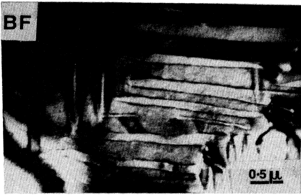
FIG. 1. Bright field micrograph of antiferroelectric phase at -170^{\circ}\text{C} in \text{PbCo}_{1/2}\text{WO}_3 .
