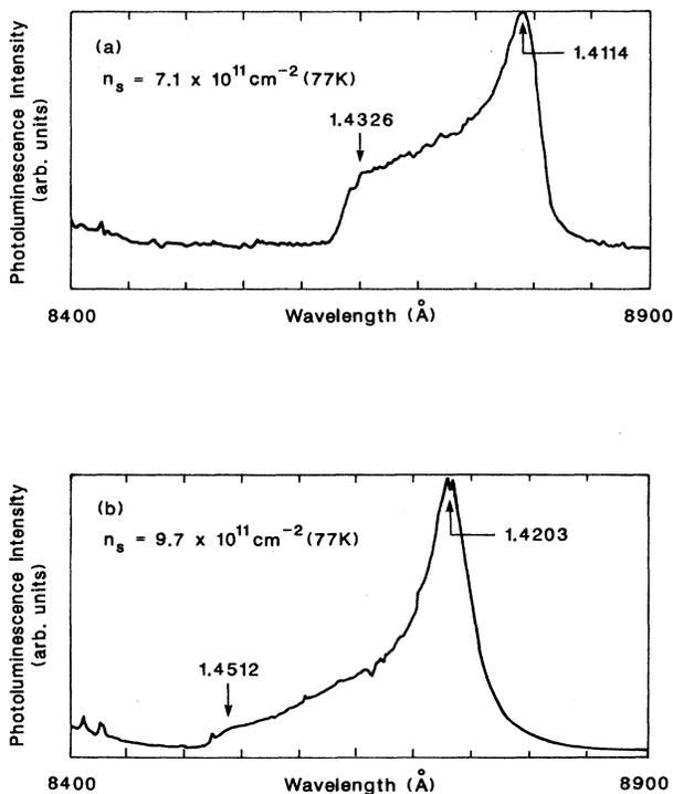
FIG. 7. Photoluminescence spectra observed from two *n*-type modulation-doped 150-Å  $\text{Al}_{0.23}\text{Ga}_{0.77}\text{As}/\text{In}_{0.11}\text{Ga}_{0.89}\text{As}/\text{GaAs}$  SQW's having differing sheet carrier concentration. (a)  $n_s = 7.1 \times 10^{11} \text{ cm}^{-2}$  (77 K). (b)  $n_s = 9.7 \times 10^{11} \text{ cm}^{-2}$  (77 K).
