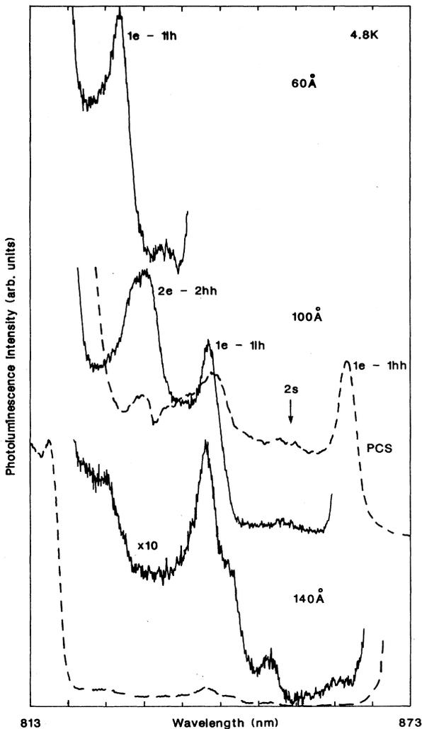
FIG. 6. Photoluminescence excitation spectrum as a function of well width in GaAs/In<sub>0.11</sub>Ga<sub>0.89</sub>As/GaAs SQW. The dashed curve for the 100-Å well is the 4.8-K photoconductivity excitation spectrum for comparison with the PLE spectrum.
