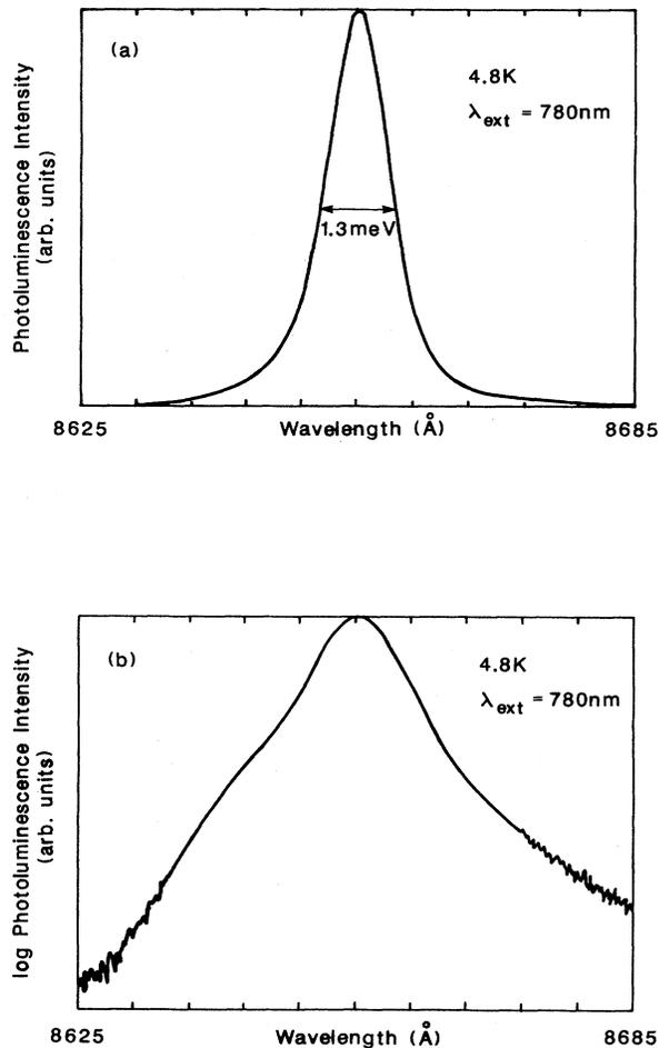
FIG. 1. Photoluminescence from 100-Å GaAs/ $\text{In}_{0.11}\text{Ga}_{0.89}\text{As}$ /GaAs SQW: (a) linear intensity scale; (b) logarithmic intensity scale.
