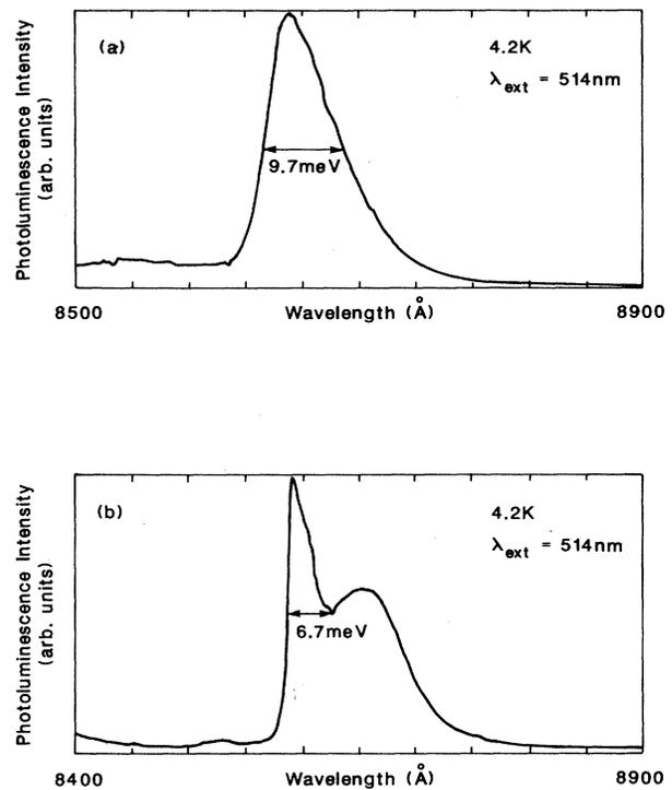
FIG. 5. Photoluminescence spectra observed in (a) 150-Å  $\text{Al}_{0.15}\text{Ga}_{0.85}\text{As}/\text{In}_{0.11}\text{Ga}_{0.89}\text{As}/\text{Al}_{0.15}\text{Ga}_{0.85}\text{As}$  SQW and (b) inverted 150-Å  $\text{GaAs}/\text{In}_{0.11}\text{Ga}_{0.89}\text{As}/\text{Al}_{0.23}\text{Ga}_{0.77}\text{As}$  SQW structure.
