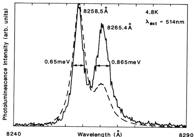
FIG. 3. Photoluminescence spectra from 20-Å GaAs/ $\text{In}_{0.11}\text{Ga}_{0.89}\text{As}/\text{GaAs}$  SQW at high (dotted line) and low excitation (solid line) intensities.
