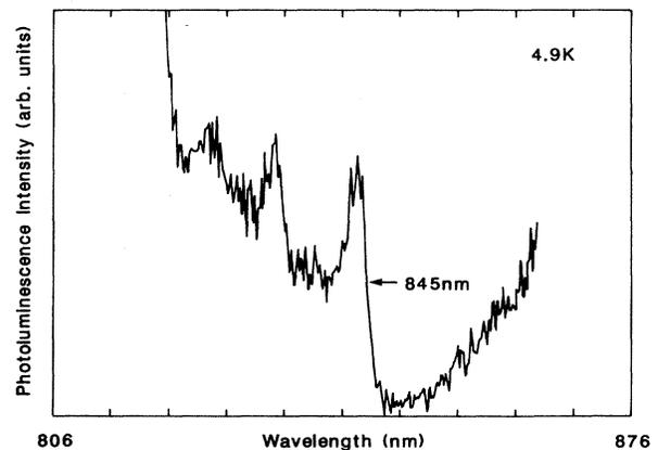
FIG. 8. PLE spectrum observed by monitoring the PL of Fig. 7(b) at 8725 Å.
