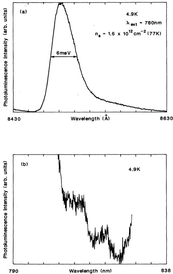
FIG. 9. (a) PL spectrum observed in  $n$ -type modulation-doped sample having a sheet carrier concentration of  $1.6 \times 10^{12} \text{ cm}^{-2}$  at 77 K. (b) PLE spectrum recorded by monitoring the PL of (a) at 8490 Å.
