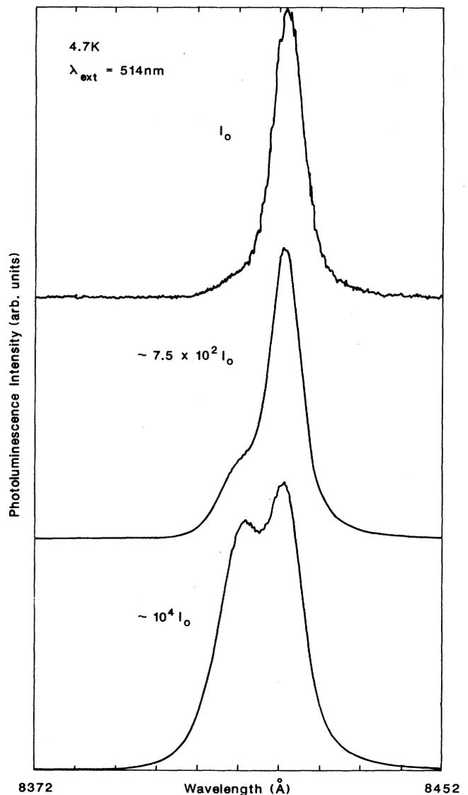
FIG. 2. Photoluminescence spectra from 60-Å GaAs/ $\text{In}_{0.11}\text{Ga}_{0.89}\text{As}$ /GaAs SQW at different excitation intensities. With increasing intensity the high-energy peak grows with respect to the lower-energy peak.
