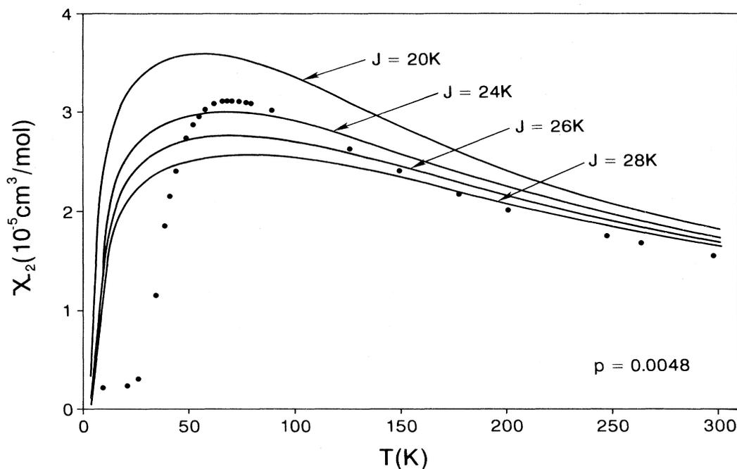
FIG. 4. Theoretical plots of the dimer susceptibility,  $\chi_2$  [Eq. (5)] vs temperature for different values of  $J$ , and the experimentally determined values of  $\chi_2$ .
