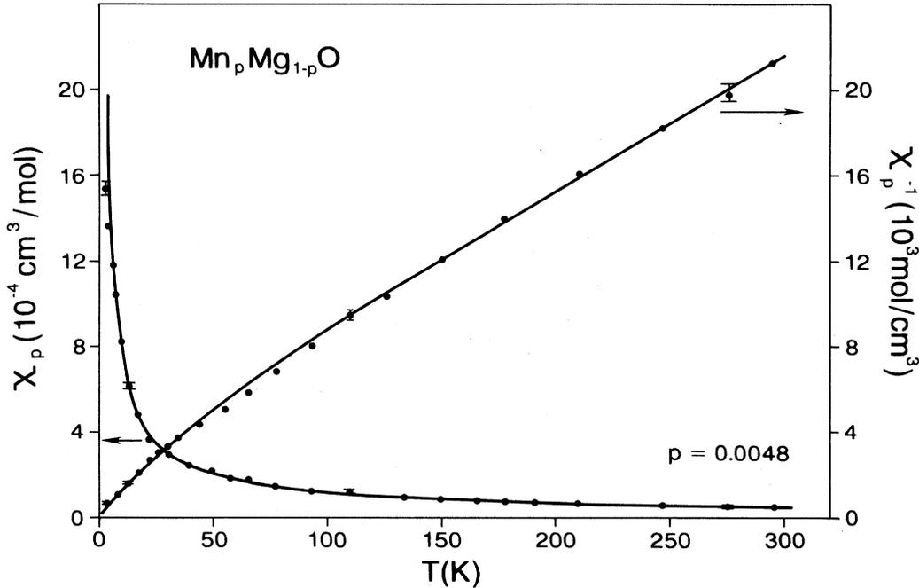
FIG. 3. Temperature dependence of the paramagnetic susceptibility,  $\chi_p$ , and that of  $\chi_p^{-1}$  for the  $\text{Mn}_p\text{Mg}_{1-p}\text{O}$  sample with nominal  $p=0.0048$ . The solid lines are theoretical fits. See text for details.
