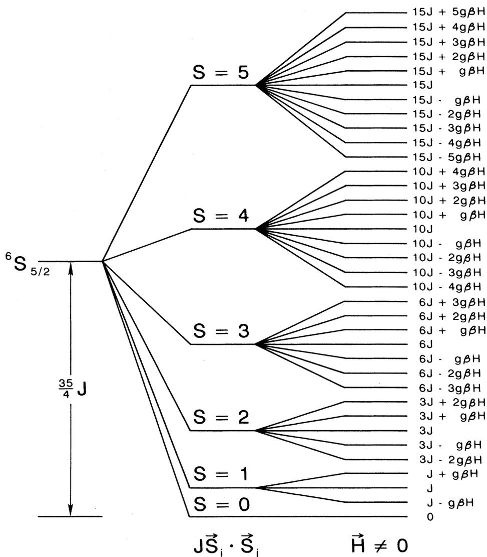
FIG. 1. Energy levels of  $Mn^{2+}$ - $Mn^{2+}$  pairs in an exchange field and in an applied field  $H$ . The zero of energy has been shifted by  $-\frac{35}{4}J$  in the Zeeman levels.
