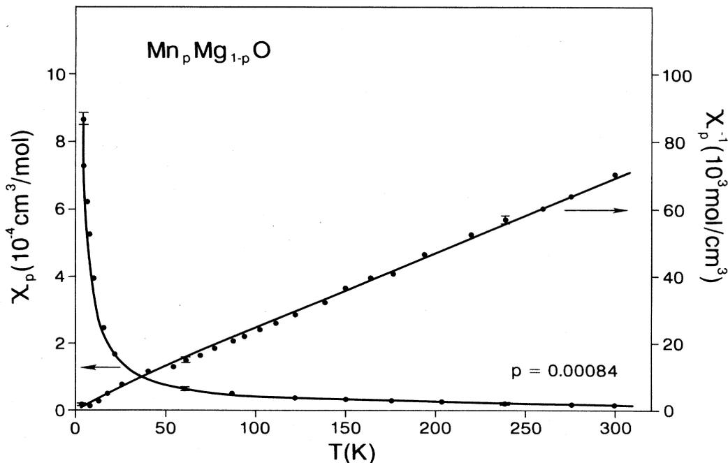
FIG. 2. Temperature dependence of the paramagnetic susceptibility,  $\chi_p$ , and that of  $\chi_p^{-1}$  for the  $\text{Mn}_p\text{Mg}_{1-p}\text{O}$  sample with nominal  $p = 0.00084$ . The solid lines are theoretical fits. See text for details.
