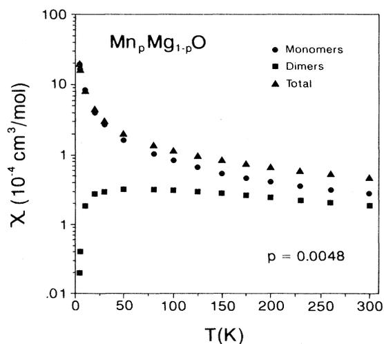
FIG. 5. Semilog plot of the susceptibility due to monomers ( $\chi_1$ ) and dimers ( $\chi_2$ ), and  $\chi_p = \chi_1 + \chi_2$  vs temperature for the higher concentration sample with  $p = 0.0048$  in  $\text{Mn}_p\text{Mg}_{1-p}\text{O}$ .
