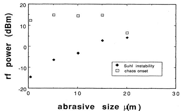
FIG. 6. rf power necessary for Suhl instability and onset of chaos in roughened YIG spheres.
