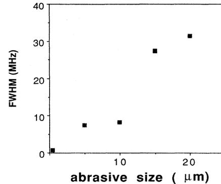
FIG. 5. Full width at half maximum of the ferromagnetic resonance line in roughened YIG spheres.
