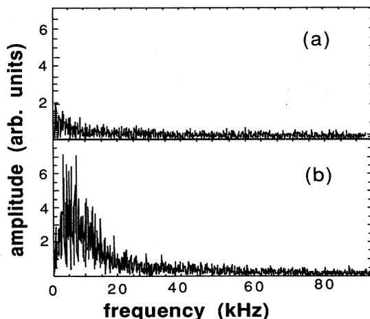
FIG. 3. (a) Fourier amplitude spectrum for chaos in a polished YIG sphere. (b) Fourier amplitude spectrum for intermittency such as that shown in Fig. 2.
