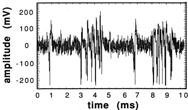
FIG. 2. Experimental time series showing bursting or intermittency in a rough YIG sphere. Measured burst interval is the time from the start of one large burst to the start of the next.
