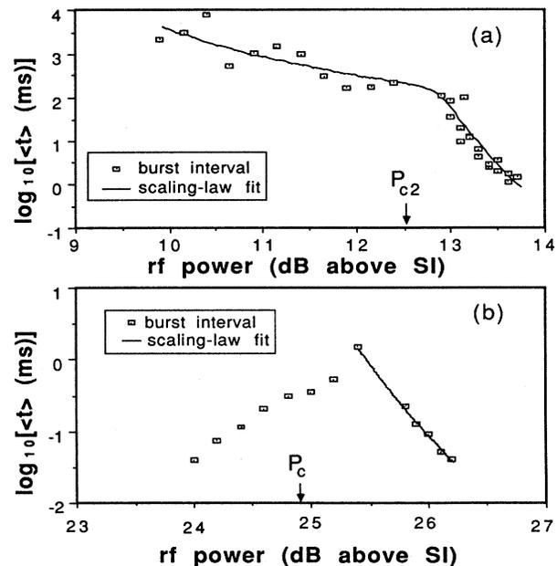
FIG. 4. (a) Average time between bursts and combined scaling law fit for intermittency at 2.5 GHz. (b) is the average time between bursts and a scaling law fit for intermittency at 2.4 GHz.
