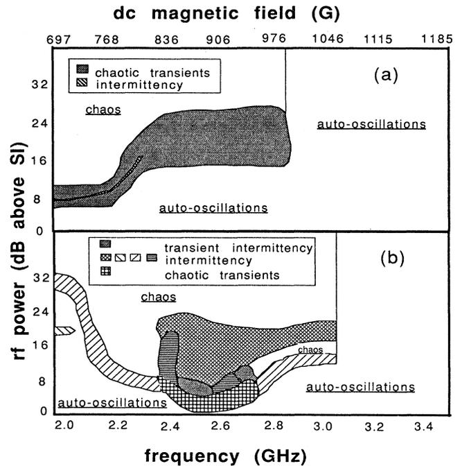
FIG. 1. Parameter space plots of the behavior of auto oscillations in YIG spheres driven at the ferromagnetic resonance frequency. (a) is for polished spheres, while (b) is for spheres roughened with  $5\text{-}\mu\text{m}$  abrasive.
