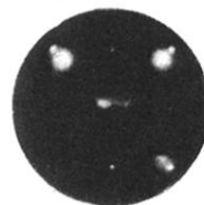
FIG. 1. (a) LEED spot pattern observed for ambient-temperature saturated oxide on Ni(001) at an incident energy of 64 eV. (The specimen holder obscures some spots from left to right across the image.) At right the positions and suggested origins of the several structures are indicated. (b) Same as (a), but after a light anneal to approximately 250°C over about 10 min.
