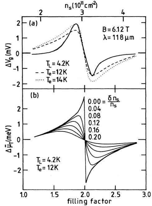
FIG. 2. (a) Photovoltage  $\Delta V_g$  measured at cyclotron resonance ( $\lambda = 118 \mu\text{m}$ ) vs Landau-level filling factor. The dashed and dotted curves are calculated gate-source potential differences as described in the text. (b) Calculated differences of the average electron chemical potentials  $\Delta\mu_T = \bar{\mu}(T_e) - \bar{\mu}(T_L)$  vs filling factor for different inhomogeneity parameters  $\delta n_s / n_s$ .
