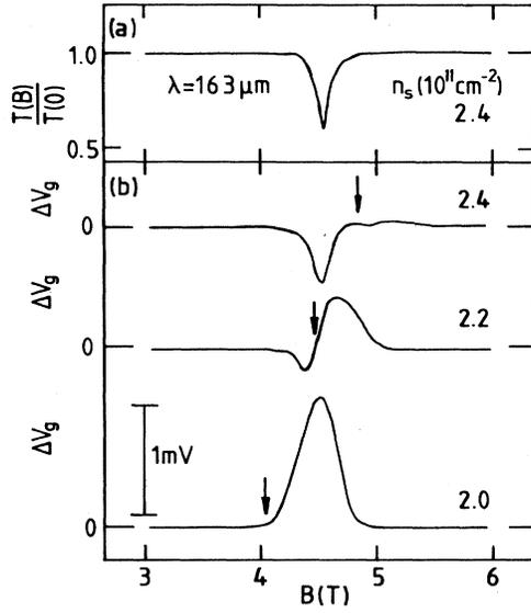
FIG. 1. (a) Cyclotron resonance at electron density  $n_s = 2.4 \times 10^{11} \text{ cm}^{-2}$  recorded in transmission  $T$ , and (b) photovoltages  $\Delta V_g$  measured at different  $n_s$ . The laser wavelength is  $\lambda = 163 \mu\text{m}$ . The arrows mark magnetic fields  $B_v = \hbar n_s / ve$  with the Landau-level filling factor  $\nu = 2$ . The lattice temperature is  $T_L = 4.2 \text{ K}$ .
