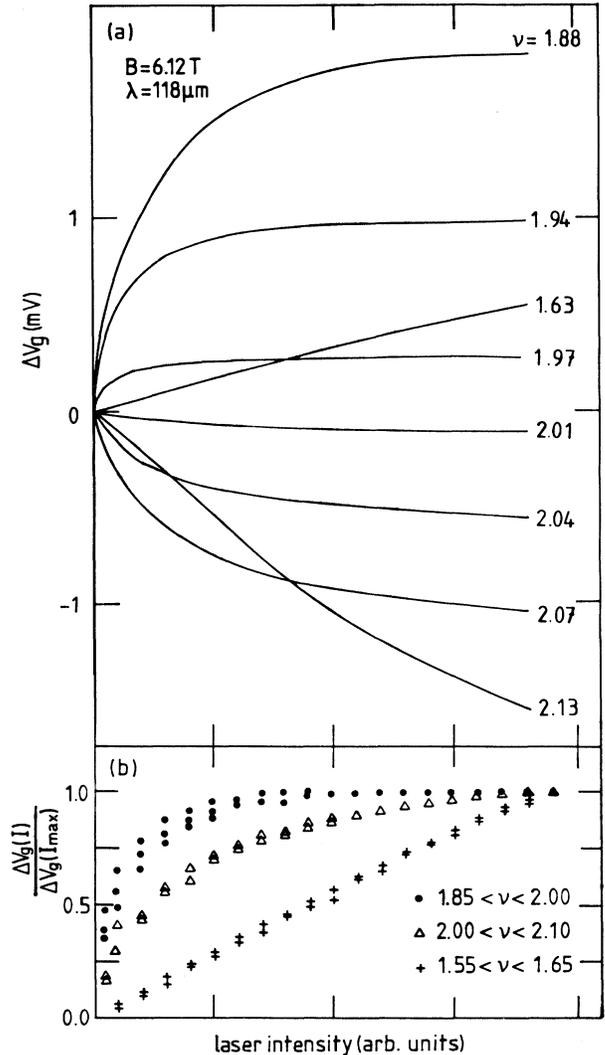
FIG. 3. (a) Dependence of the photovoltage on FIR laser intensity at various Landau-level filling factors close to  $\nu=2$ . (b) Normalized photovoltages  $\Delta V_g(I)/\Delta V_g(I_{\max})$  vs laser intensity for different filling factor regimes.
