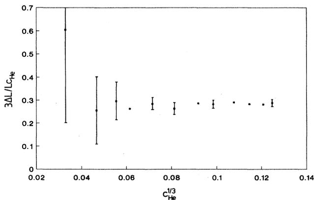
FIG. 4.  $3\Delta L/(Lc_{\text{He}}) \approx \Delta V/(Vc_{\text{He}})$  vs  $c_{\text{He}}^{1/3}$  for  $\text{NbT}_{0.0253}$ .
