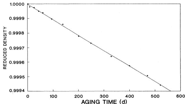
FIG. 1. Reduced density of  $\text{NbT}_{0.0253}$ ,  $\rho(t)/\rho(0)$ , vs aging time. The density of the tritide was measured using a high-precision buoyancy technique (Ref. 16). The straight line represents a linear least-squares fit.
