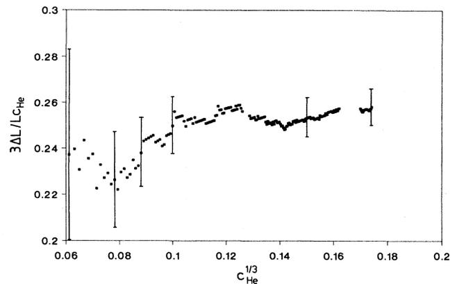
FIG. 5.  $3\Delta L/(Lc_{\text{He}}) \approx \Delta V/(Vc_{\text{He}})$  vs  $c_{\text{He}}^{1/3}$  for  $\text{TaT}_{0.0744}$ .
