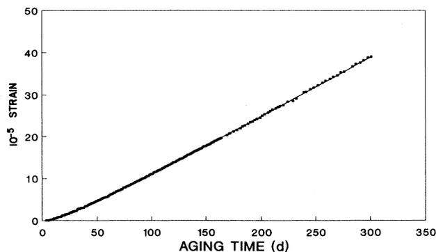
FIG. 3. Relative length change of a  $\text{LuT}_{0.15}$  sample vs aging time as measured at  $-195^\circ\text{C}$  using strain gauges with known  $k$  factors at that temperature.
