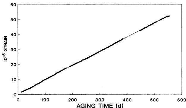
FIG. 2. Relative length change of  $\text{TaT}_{0.0774}$  vs aging time as measured at room temperature with strain gauges.
