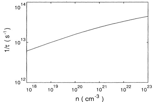
FIG. 3. The maximum scattering rate from electron-hole collisions as a function of density. The results are valid for an electron-hole plasma in the model semiconductor described in the text.
