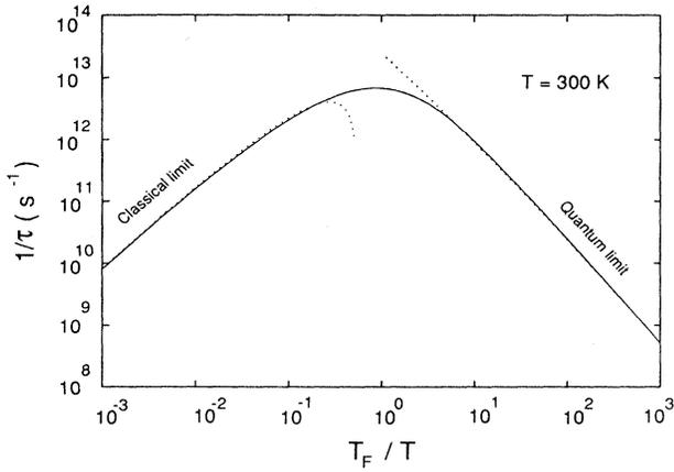
FIG. 1. The scattering rate from electron-hole collisions as a function of  $T_F/T$ . The results are valid for an electron-hole plasma at  $T=300$  K. The solid curve is the result from the present approach. The dotted curves are the results from the Boltzmann approach, as obtained in Ref. 2, in the classical and quantum limits. The quantum-limit result has been modified (see the main text).
