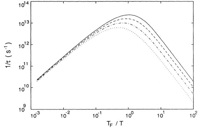
FIG. 2. The scattering rate from electron-hole collisions as a function of  $T_F/T$ . Each curve is valid for an electron-hole plasma at fixed density. The dotted, dash-dotted, dashed, and solid curves are for the plasma densities  $1 \times 10^{18}$ ,  $1 \times 10^{19}$ ,  $1 \times 10^{20}$ , and  $1 \times 10^{21} \text{ cm}^{-3}$ , respectively.
