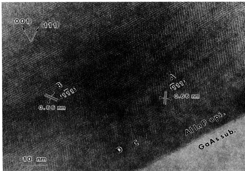
FIG. 1. Lattice image of \text{Al}_{0.5}\text{In}_{0.5}\text{P} for [110] electron beam incidence. T_g = 700^\circ\text{C} . c^{\text{V}}/c^{\text{III}} = 180 .
