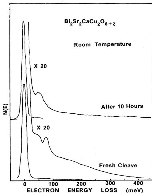
FIG. 1. Electron energy-loss spectra of  $\text{Bi}_2\text{Sr}_2\text{CaCu}_2\text{O}_8$  cleaved at room temperature, immediately after cleaving and 10 h later. The primary energy was 8 eV and the electrons were incident at  $60^\circ$  from the surface normal.
