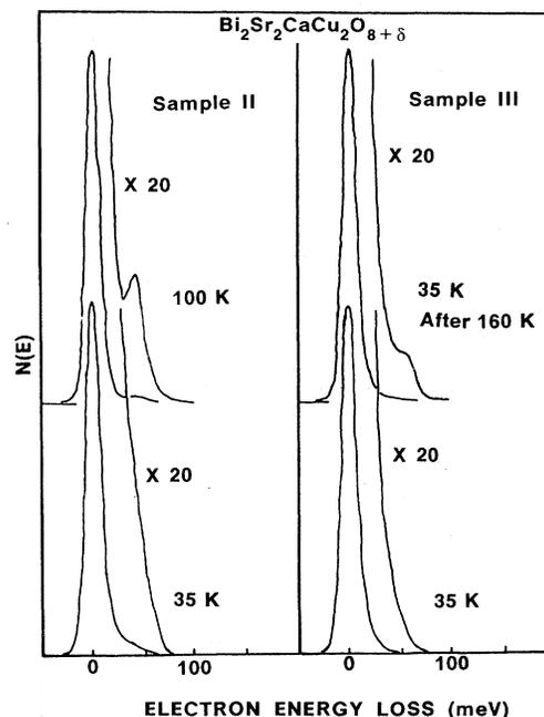
FIG. 2. Electron energy-loss spectra from  $\text{Bi}_2\text{Sr}_2\text{CaCu}_2\text{O}_8$  cleaved at 35 K, and after warming above 110 K. These spectra are representative, but the intensities of the features showed significant variation in the course of our experiments.
