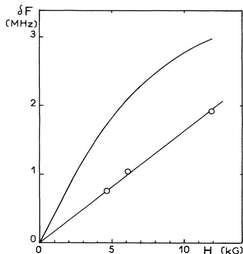
FIG. 3. Line shift at 1.8 K as a function of applied magnetic field. The upper curve is calculated for an uncoupled system deduced from the Brillouin function  $B_{7/2}(7\mu_B H/1.8k)$  (see text).
